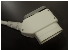
Figure 1-1 Photograph of a P-connector
