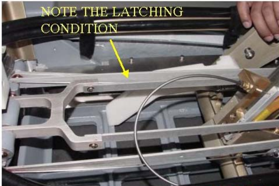
ENGAGING SAFETY LATCH BAR
