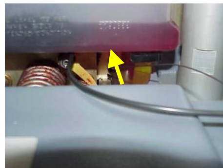
Insert the inner wire of the centre pin cable through the opening at the bottom of the oil reservoir as shown
