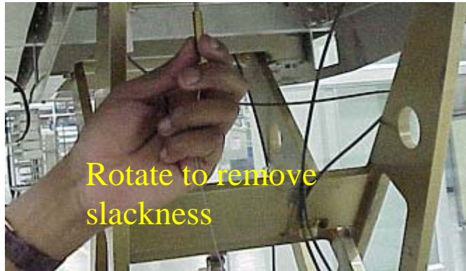
REMOVING SLACKNESS IN UP LIMIT CABLE
