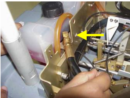
Insert the cable from bottom of the hose connector as shown and pull the wire from the front end of the lower base assembly of the table as shown.
