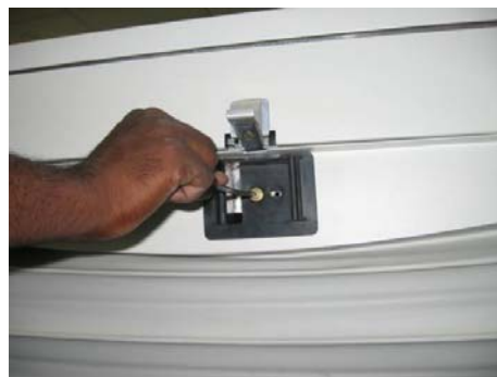
Remove latch support cover from tabletop by unscrewing the Allen screws
