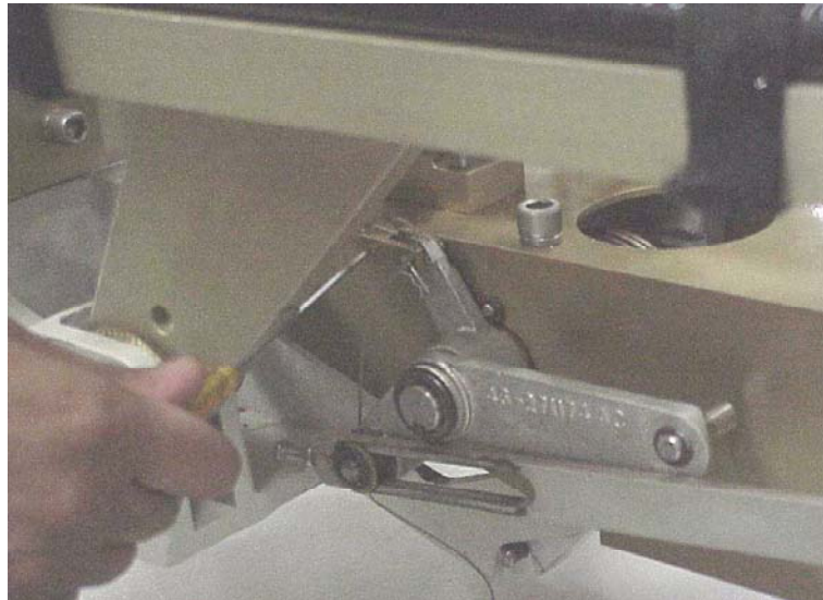
REMOVAL OF CRADLE LATCH CABLE
