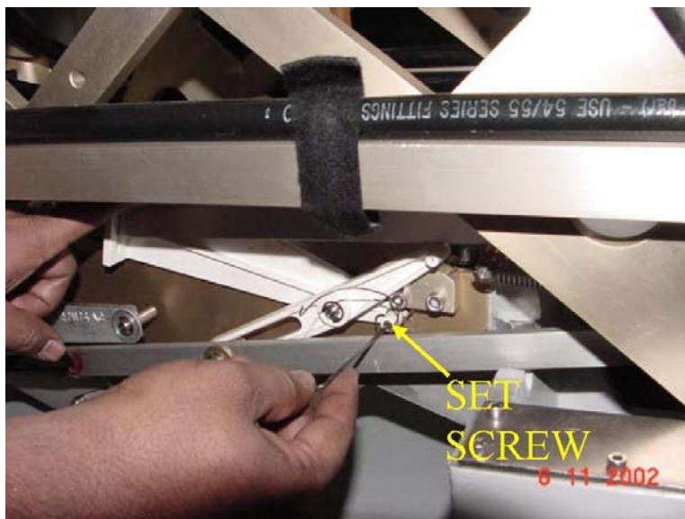
REMOVAL OF FLIPPER CABLE
