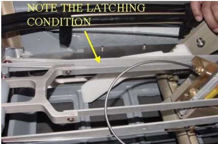
ENGAGING SAFETY LATCH BAR
