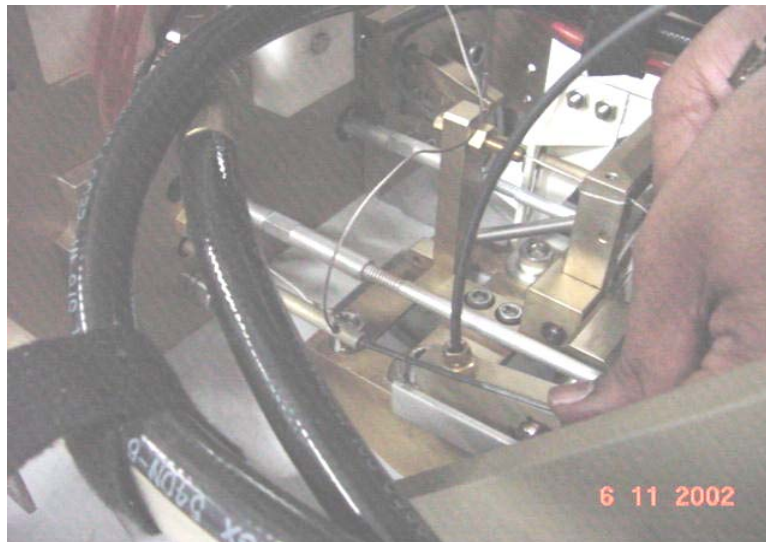
REMOVAL OF SECONDARY CRADLE LATCH ACTUATING CABLE
