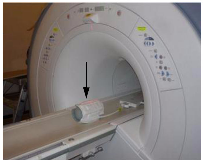
Figure 2-1 Landmarking the 16-L array (3.0T array shown) on the left and the 16-S or 16-M array on the right
