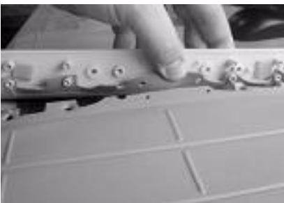
Figure 3-12 Alignment of bosses and posts in lower spine
