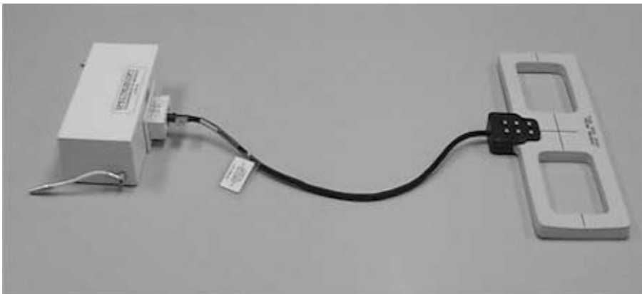
( 31 P) Phosphorus Transmit/Receive Flex Coil, MNS Q.D. BOX, and ( 31 P) Spectroscopy TR Module ILLUSTRATION 1–1
