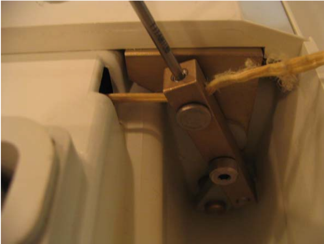
CRADLE RELEASE ADJUSTMENT ILLUSTRATION 3-26
