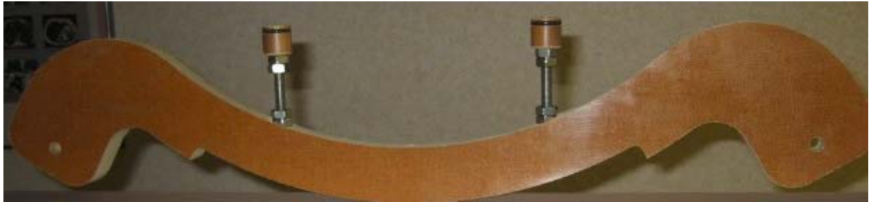
ILLUSTRATION 3-2 PHENOLIC BRIDGE SUPPORT – M10 x 30mm HEX HEAD SCREWS SEATED
