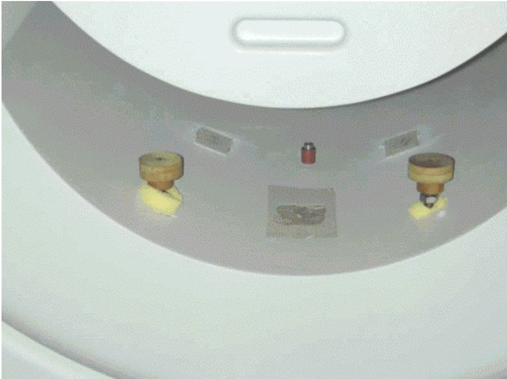
ILLUSTRATION 5-5 END BELL WITH PROPERLY FITTED ACCESS HOLE
