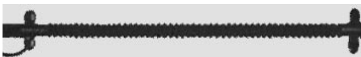
Stretching the bellows too tight results in the gain set too high.
