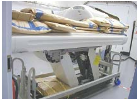
Figure 1-39 Remove Table Packing
