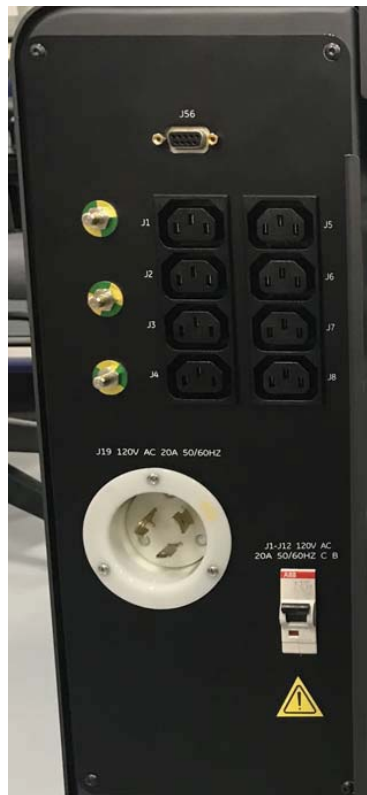
Figure 2-14 Open Console AC Box Connections
