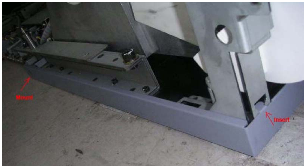
Figure 4-13 Installing Skirt Cover
