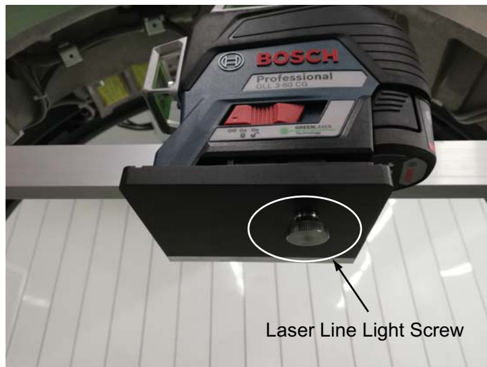
Figure 1-63 Fix the Line Laser
