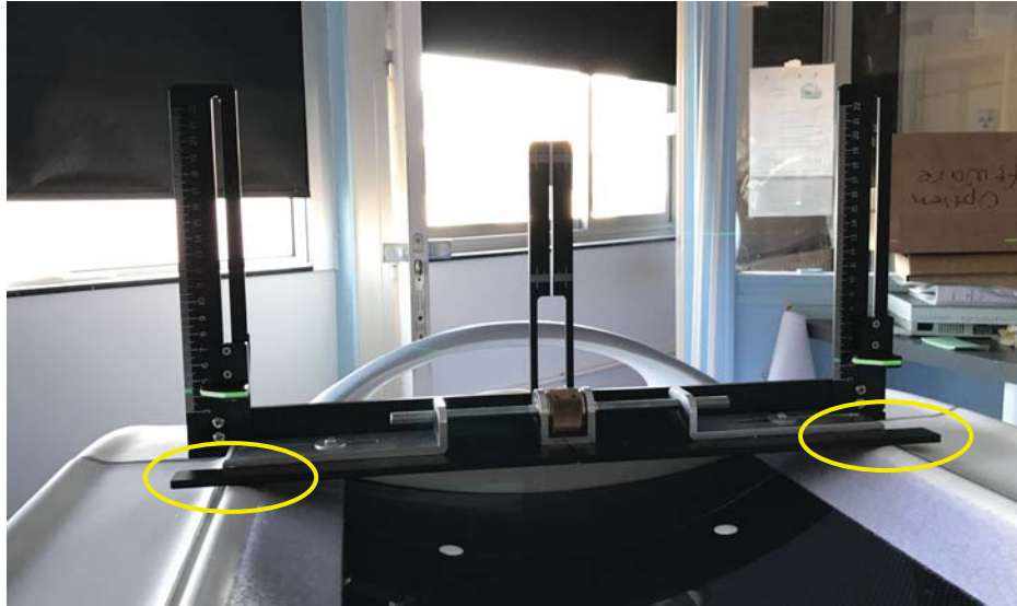
Figure 1-64 Table Alignment Tool
