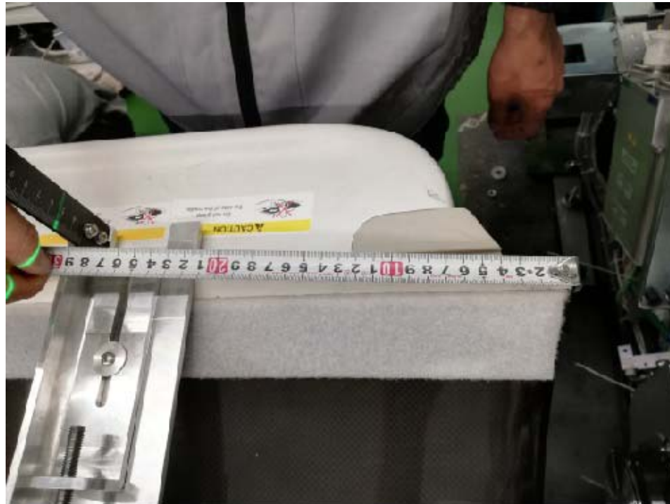
Figure 1-65 25cm Distance from Cradle Front End
