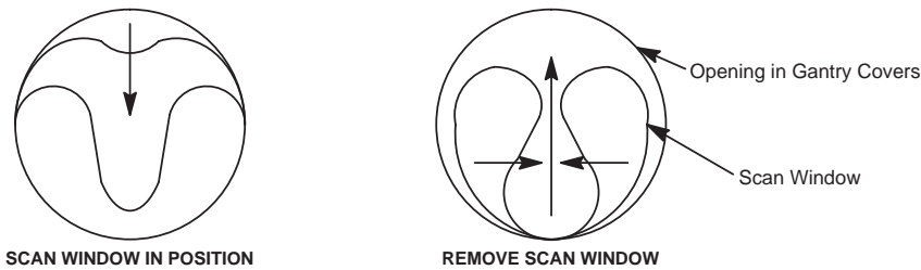
Figure A-1 Scan Window Removal
