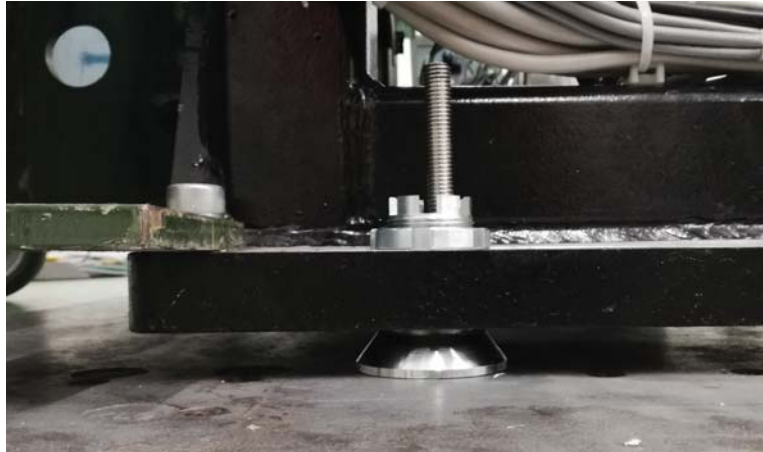
Figure 1-30 Lower the Gantry
