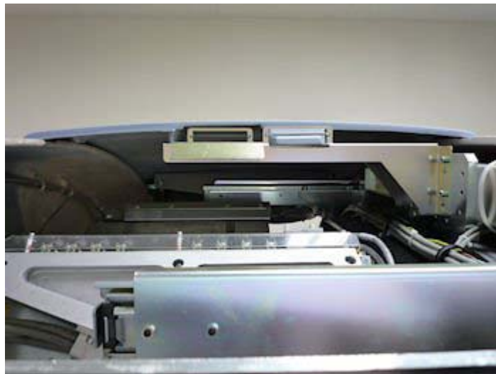
Figure A-7 Top Cover Tabs and Bracket
