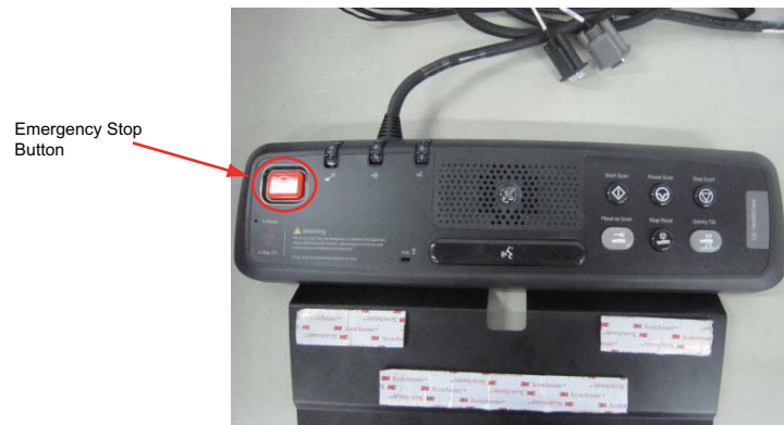
Figure 4-21 GSCB Emergency Stop Button
