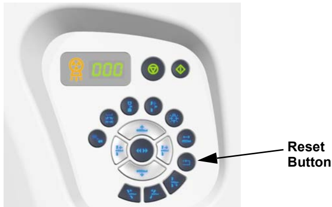
Figure 4-19 Reset buttons on Gantry Switch
