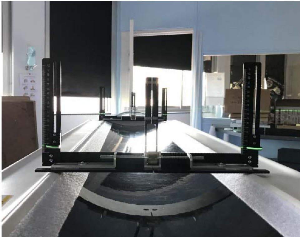
Figure 1-51 Table Alignment in X-axis and Z-axis
