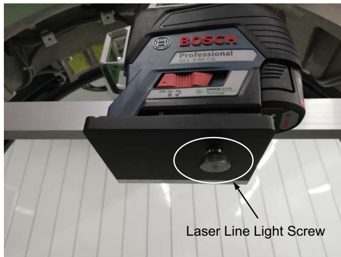
Figure 1-48 Fix the Line Laser
