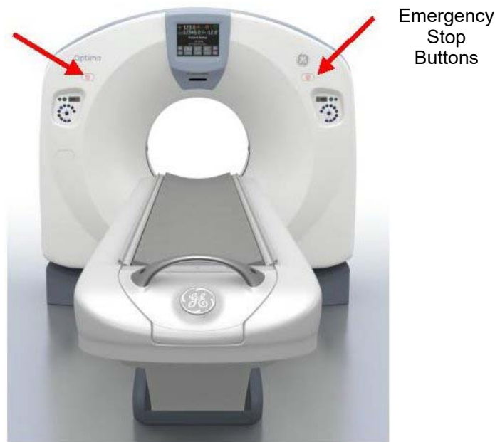
Figure 4-20 Gantry Emergency Stop Button Positions
