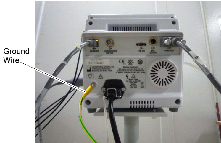
Figure 2-21 Connections on Rear of Cardiac Monitor (IVY7800)
