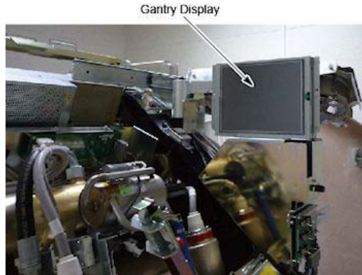
Figure A-23 Gantry Display Service Mounting Location
