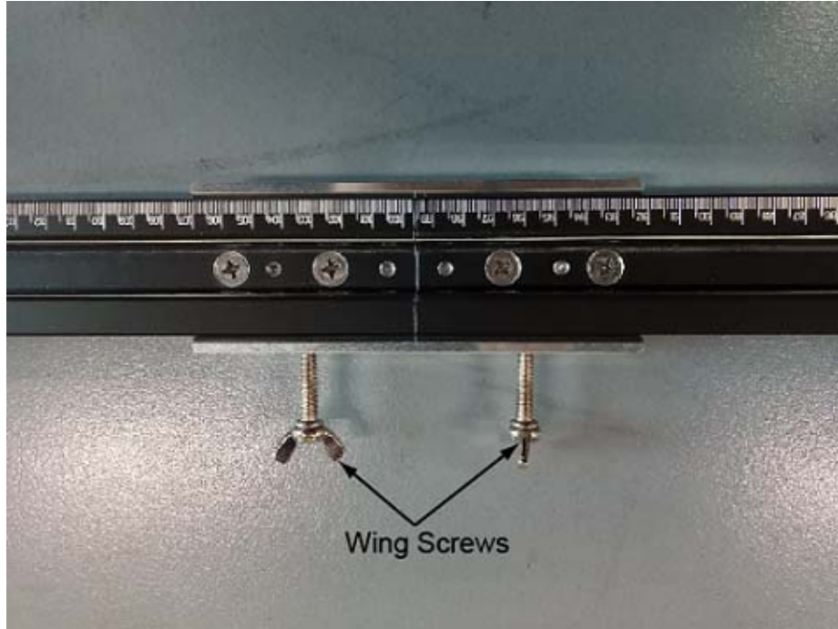
Figure 1-12 Assemble Sliding Rails
