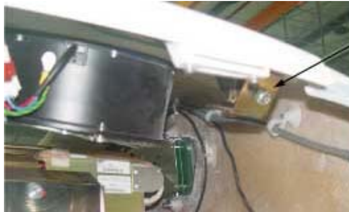
Figure A-6 Screws Securing Top Cover
