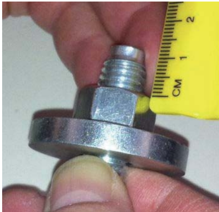
Figure 1-69 Anchor Preparation-set nut at 13.0 mm
