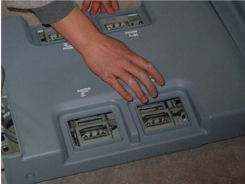
Figure 1-84 Install Front Bottom Cover
