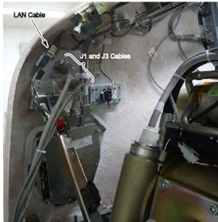
Figure A-13 Front Cover Cables
