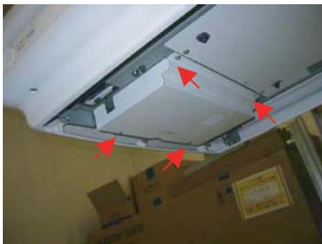
Figure 1-56 Remove Bottom Cover
