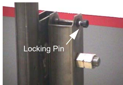
Figure A-17 releasing Front Cover Dolly Hinge
