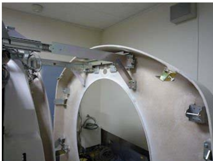
Figure A-32 Rear Cover Unlatch
