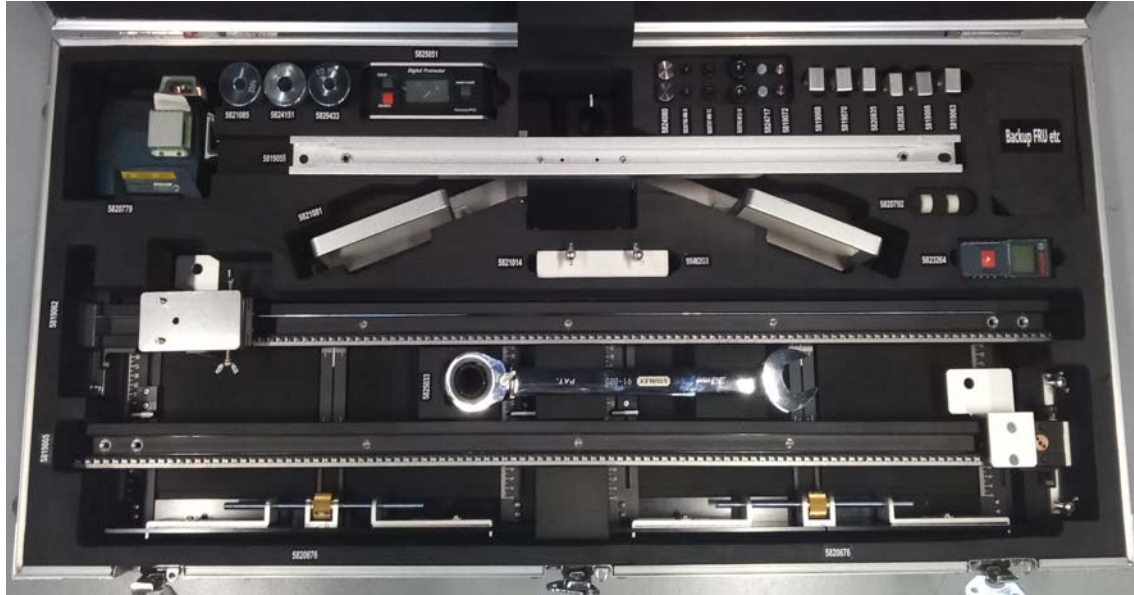
Figure 1-1 CT Installation and Alignment Tool (GE P/N: 5824714 or Equivalent)
