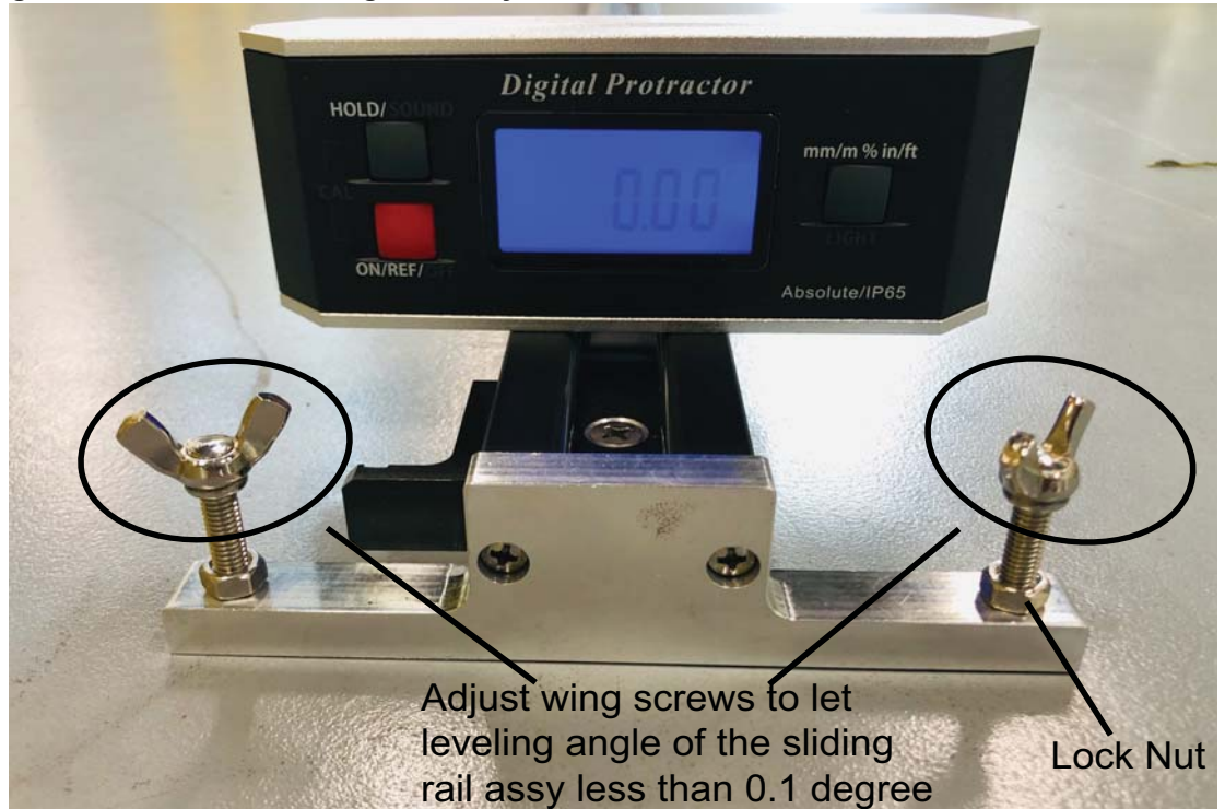
Figure 3-12 Level the Sliding Rail Assy
