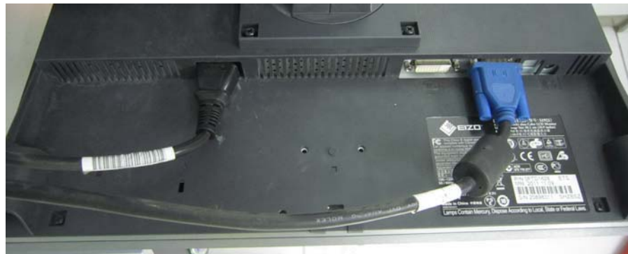
Figure 2-8 Video Cable and Power Cable
