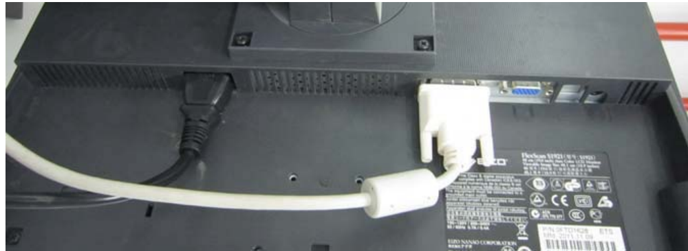
Figure 2-7 Video Cable and Power Cable
