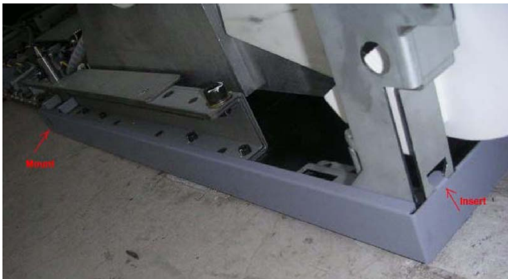
Figure 4-19 Installing Skirt Cover
