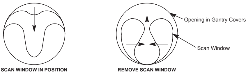
Figure A-1 Scan Window Removal
