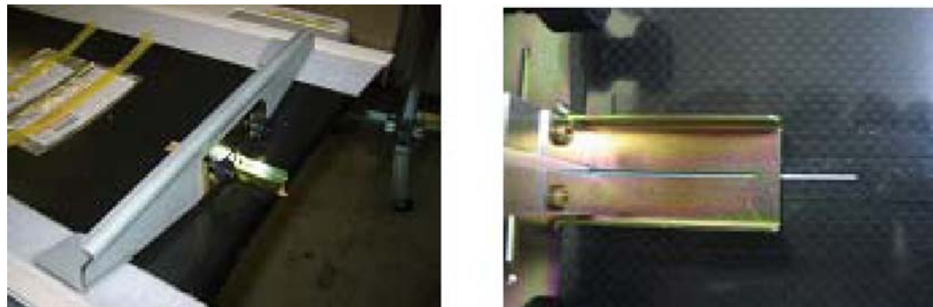
Figure 1-46 Front Table Laser Alignment
