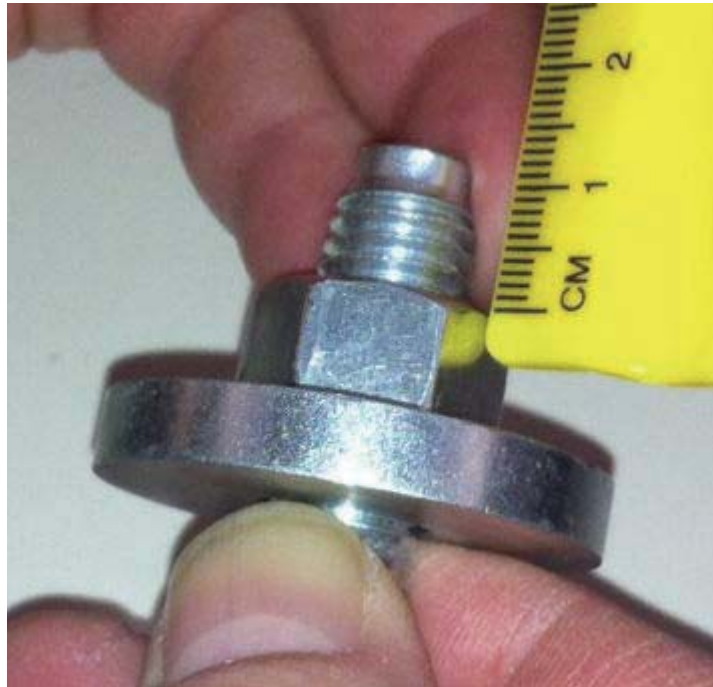
Figure 1-57 Anchor Preparation-set nut at 13.0 mm
