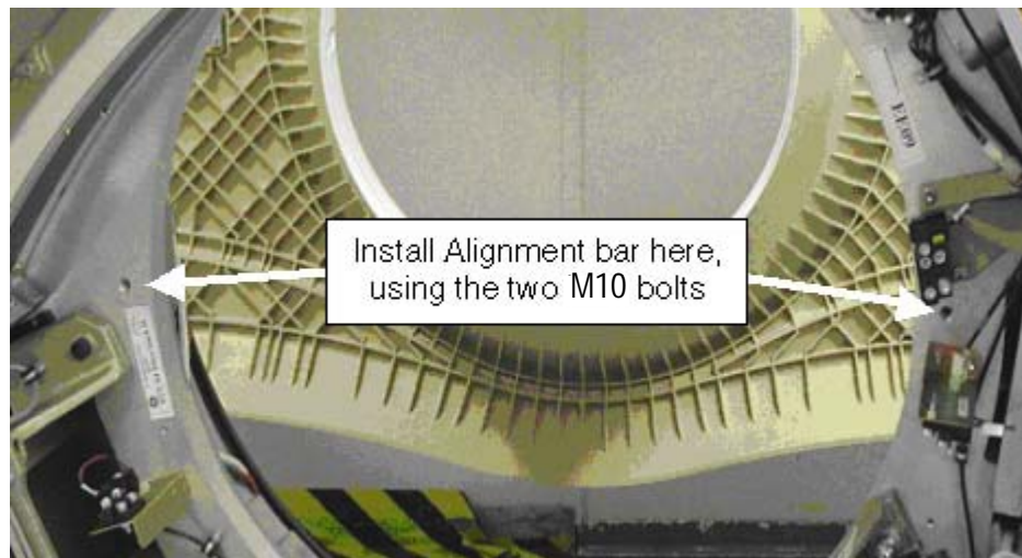
Figure 1-22 Alignment Bar Installation Location
