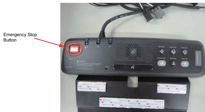
Figure 4-27 GSCB Emergency Stop Button
