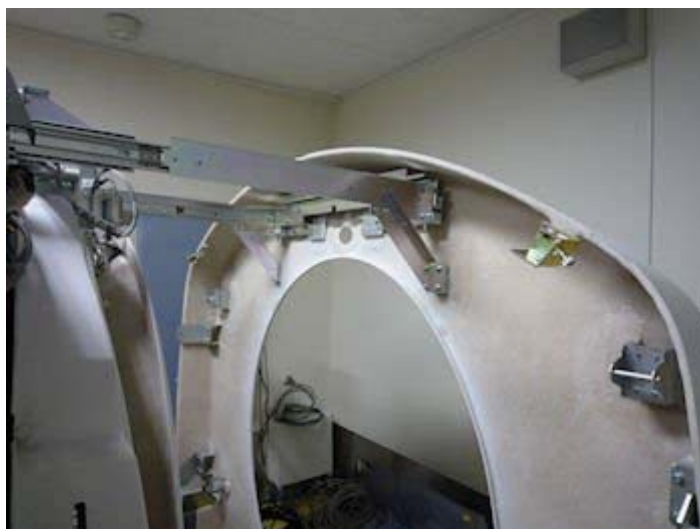
Figure A-32 Rear Cover Unlatch
