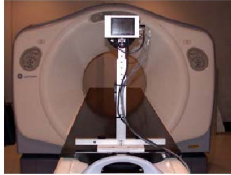
FIGURE 5-1: TYPICAL CAMERA MOUNTED ON FLAT TABLE TOP
