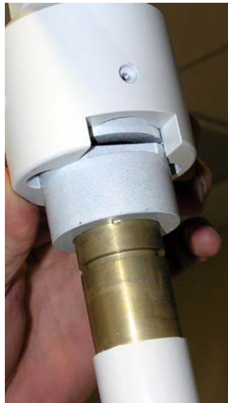
Figure 2-14 Install LCD Monitor Post
