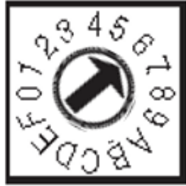
Figure 2-34 Switch to Pin 6
