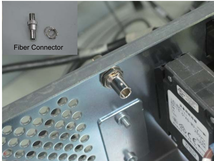
Figure 2-43 Fiber Connector Installation
