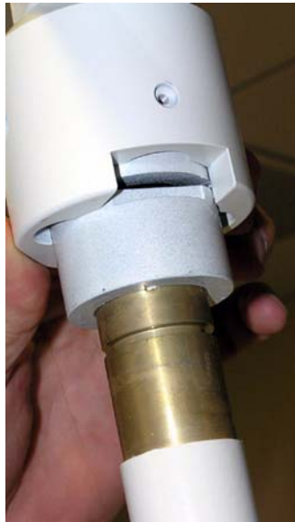
Figure 2-11 Install LCD Monitor Post
