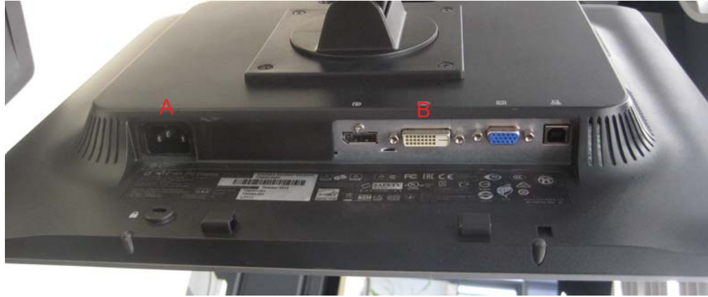
Figure 2-10 Monitor Cables for Z8G4
