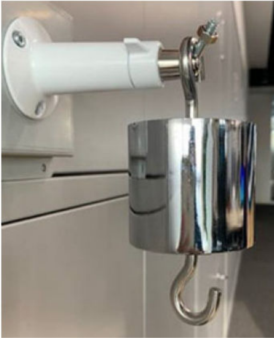
Figure 3-2 Capacity load for camera bracket
