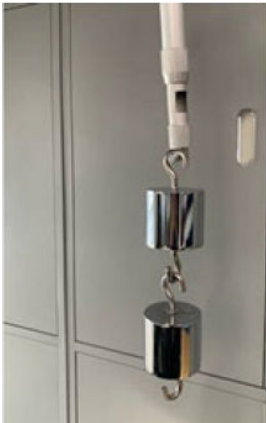
Figure 3-6 Capacity load for extendable pipe
