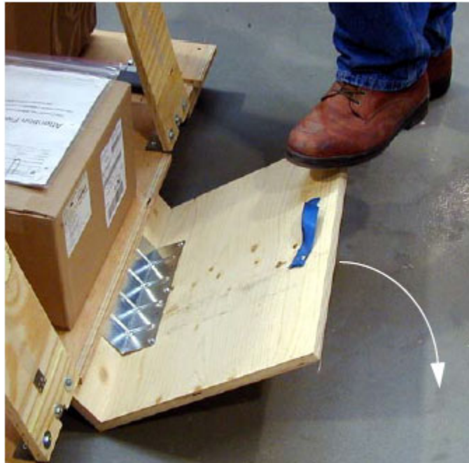
Figure 1-62 Step-board used to raise front edge of skid
