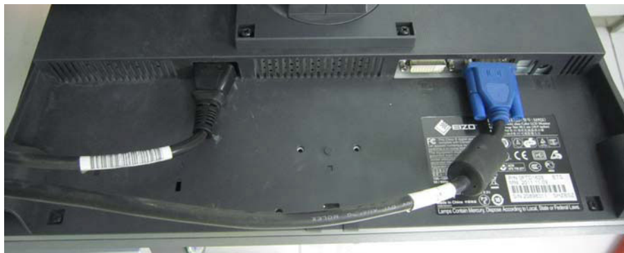
Figure 3-9 Video Cable and Power cable for Image Monitor
