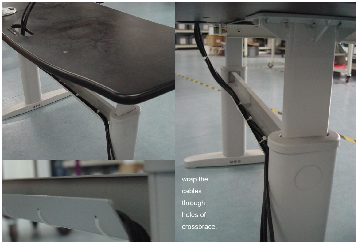
Figure B-22 Cable Routing
