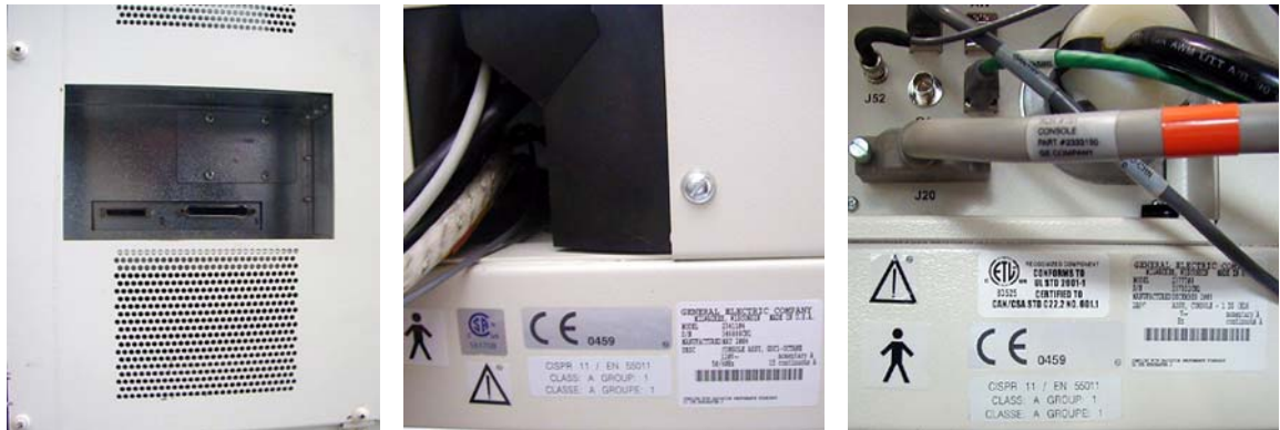
Figure 5-2 Operator Console Rating Plate Attachment (Left to Right: H3, GOC1 & GOC5) NOT Shown: GOC6-rating plate located on bottom of console in similar location as GOC5.
