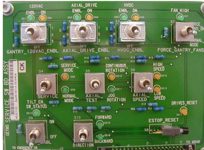
Figure 4-2 LightSpeed Gantry Service Switches
