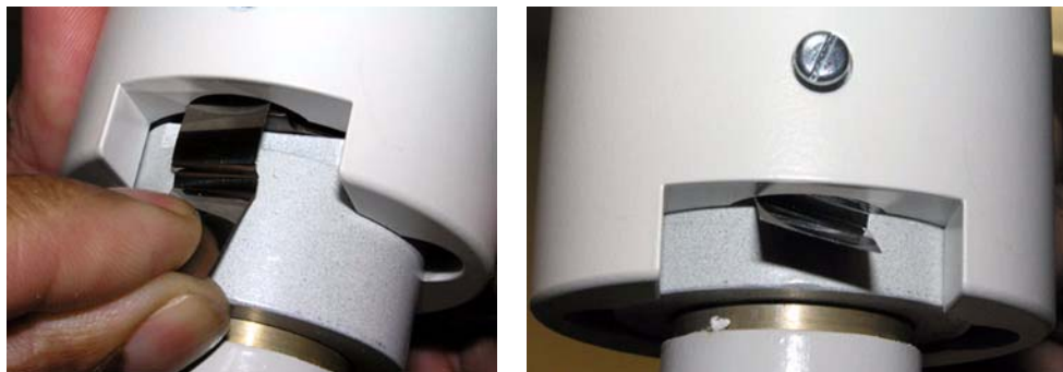
Figure 2-12 Locking Tab and Screw
