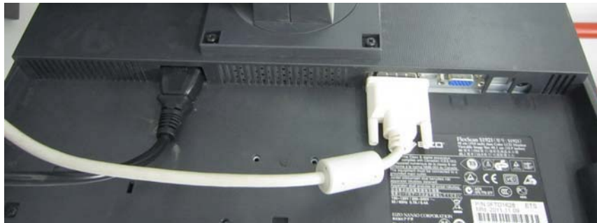
Figure 2-10 Video Cable and Power Cable
