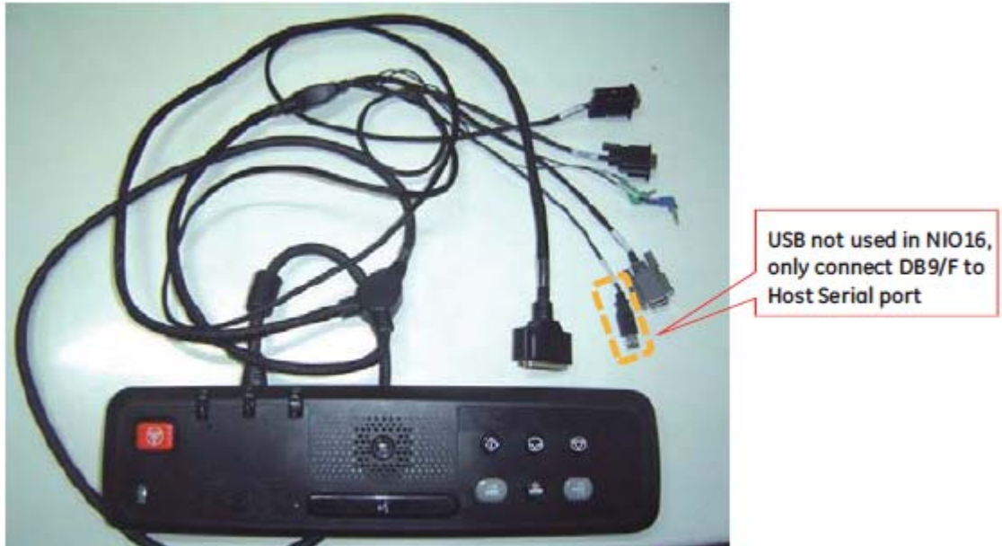
Figure 2-9 GSCB and Cable
