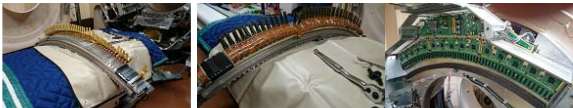
Overview of dismantled detector and DAS/Det chassis.
