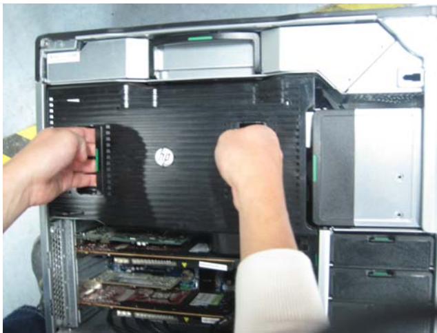
Figure 2-38 Remove the Protect Covers
