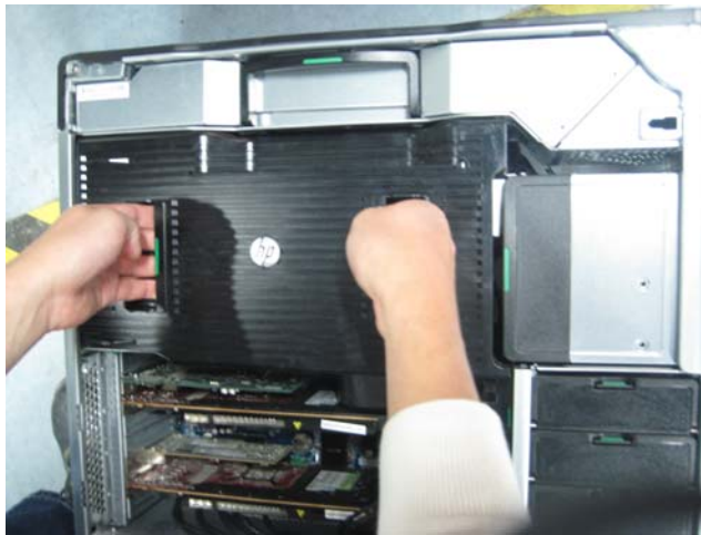
Figure 2-26 Remove the Protect Covers
