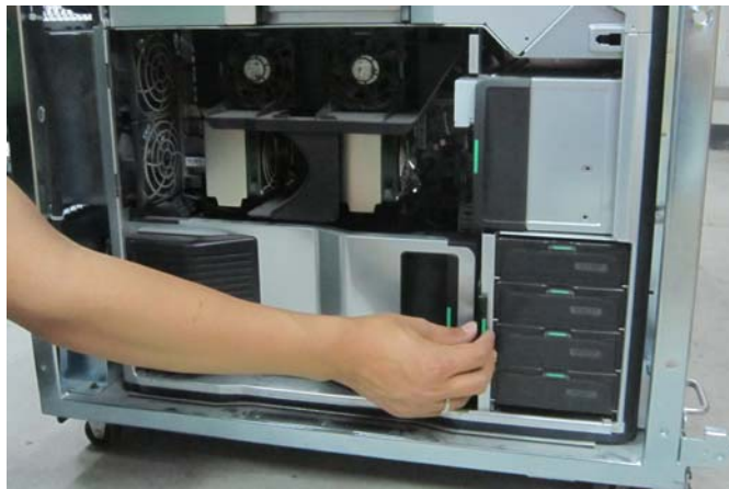
Figure 2-14 Remove the Protect Covers
