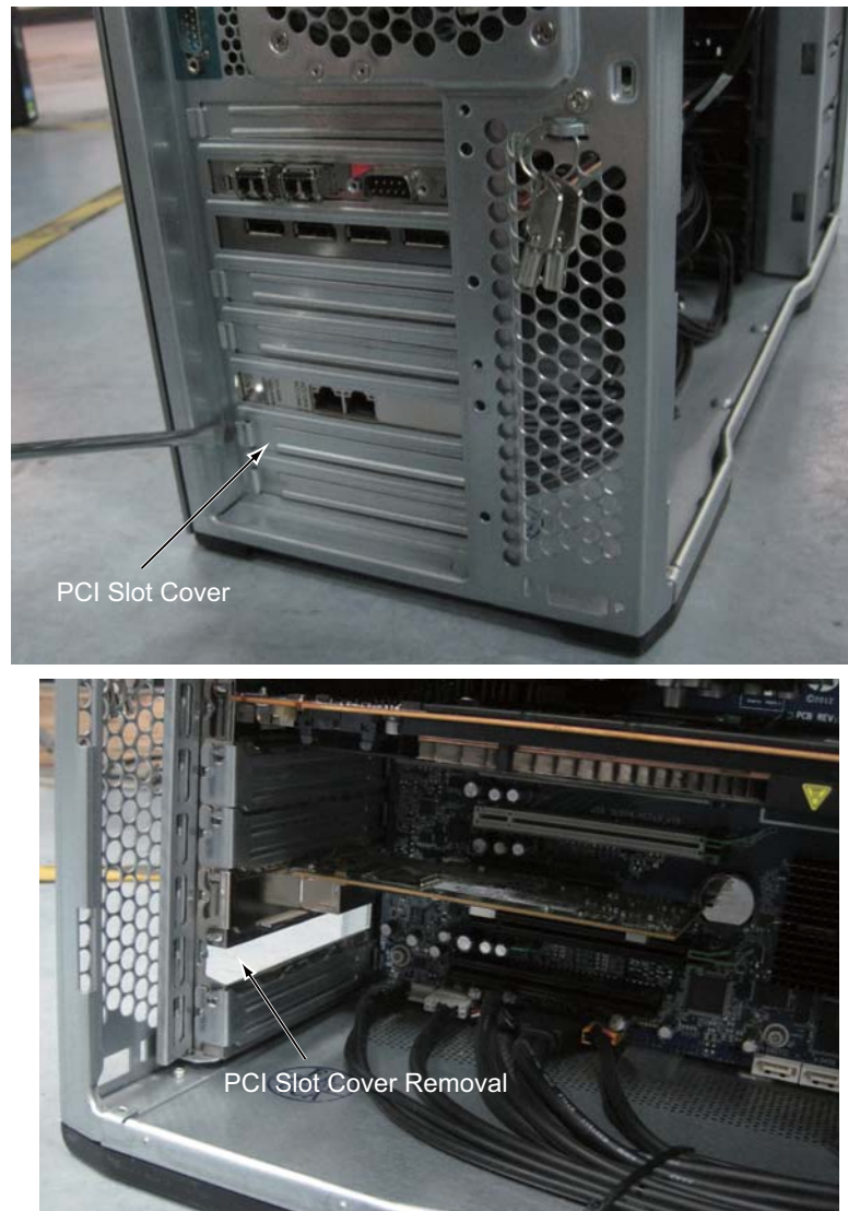
Figure 2-30 PCI Slot Cover Removal
