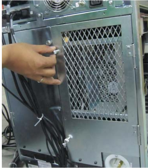
Figure 2-40 Open Back Side Cover
