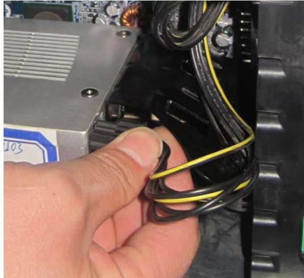
Figure 2-21 Connect Local Power
