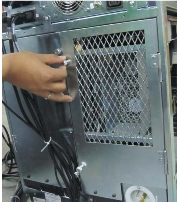
Figure 2-28 Open Back Side Cover
