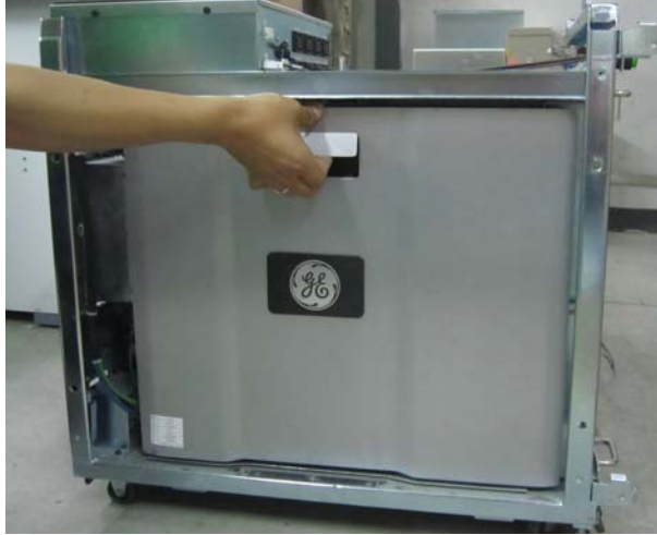
Figure 2-24 Left Side Cover
