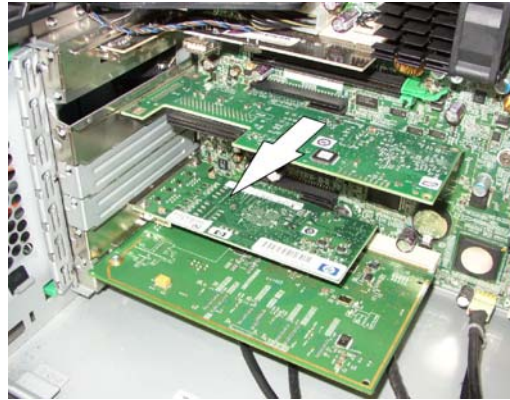
Figure 2-5 SCSI Card Removal
