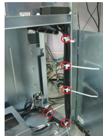
Fix DVI Video Cable (IN) on OC Chassis
