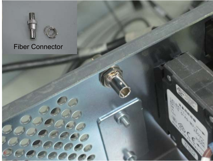
Figure 2-43 Fiber Connector Installation
