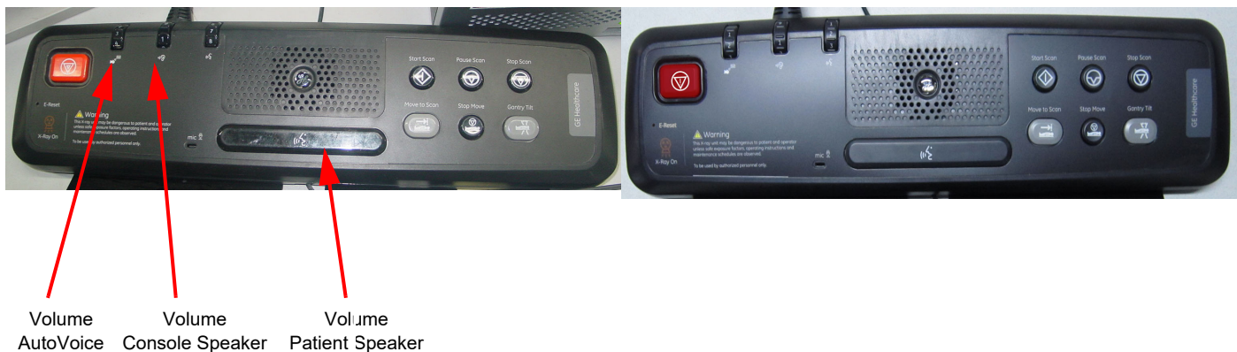
Figure 5-28 GSCB Volume Controls on NIO16 / OpenOC16 Console
