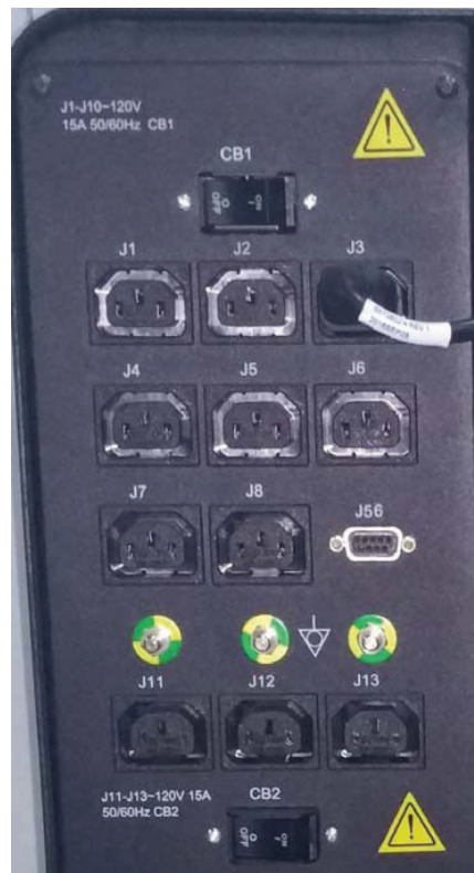
Figure 2-60 OpenOC16 Console AC Box
