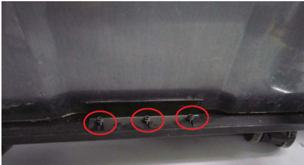
Figure 1-74 Side Access Panel
