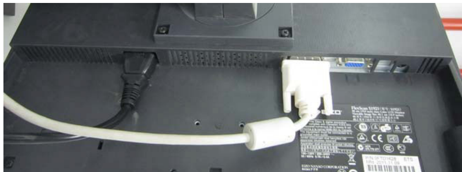
Figure 2-25 Video Cable and Power Cable
