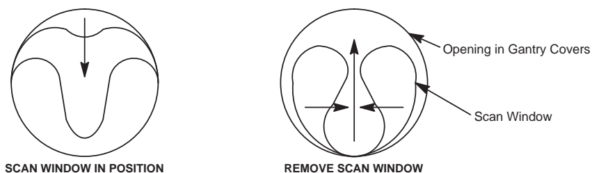
Figure A-28 Scan Window Removal
