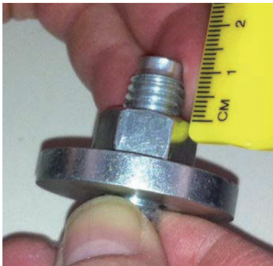
Figure 1-43 Anchor Preparation-set nut at 13.0 mm
