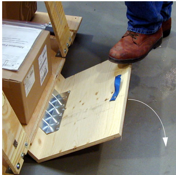
Figure 1-68 Step-board used to raise front edge of skid
