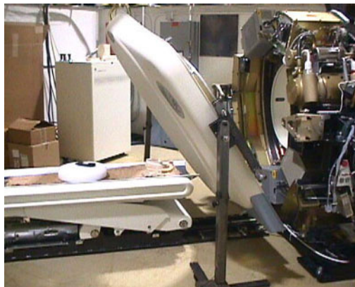
Figure A-12 Front Cover Removal Sequence
