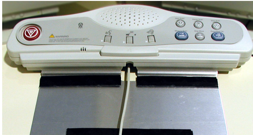
Figure 2-3 SCIM control with keyboard cable routed through SCIM
