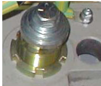
Figure 1-47 Table Base Anchor Assembly
