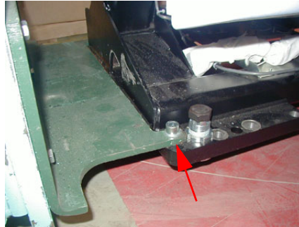
Figure 1-8 Gantry Dolly Bolts
