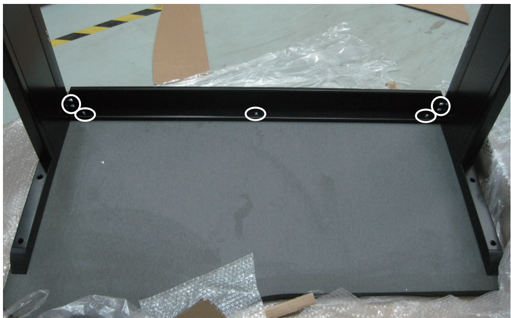
Figure B-26 Crossbar Installation
