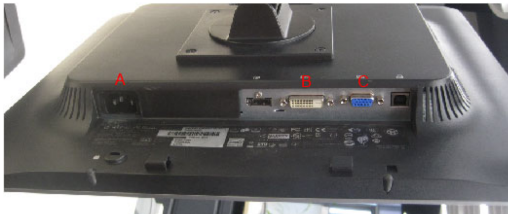
Figure 2-28 HP E190i LCD Monitor Connections
