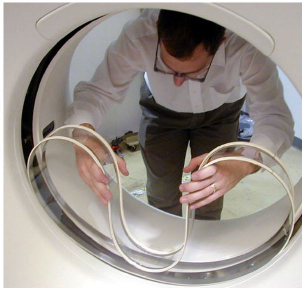
Figure A-24 Installing the mylar window
