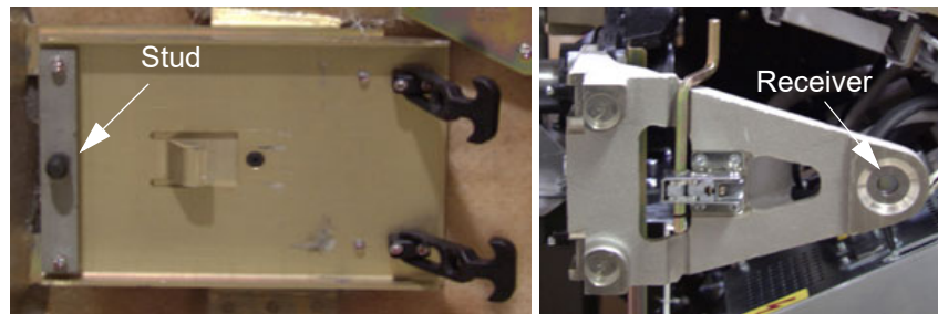
Figure A-18 Cover stud and Mounting bracket receiver
