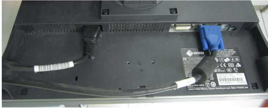
Figure 3-10 Video Cable and Power cable
