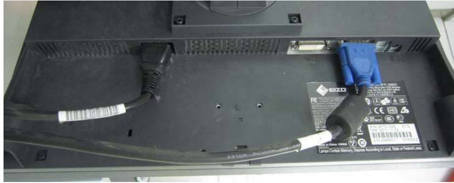
Figure 2-10 Video Cable and Power cable
