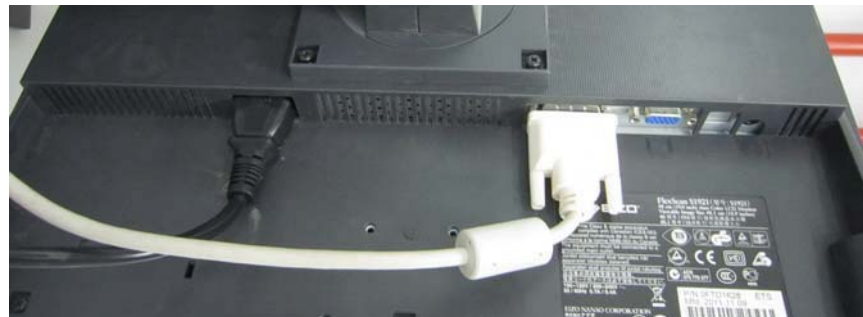
Figure 3-9 Video Cable and Power Cable
