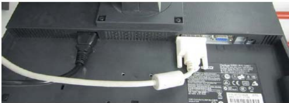
Figure 2-16 Video Cable and Power Cable for LCD Monitor
