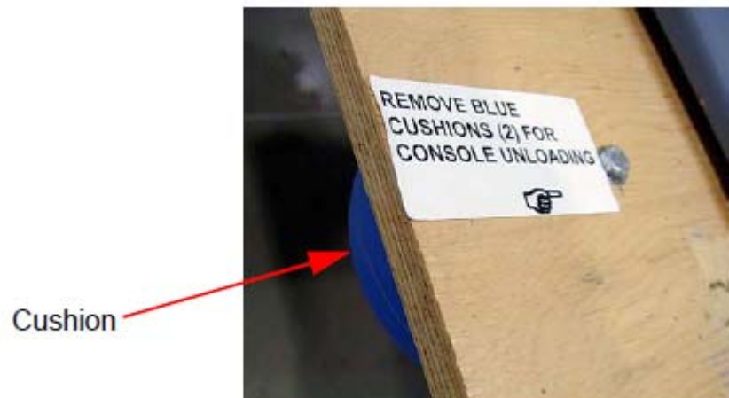
Figure 2-8 Cushion on Bottom of Skid
