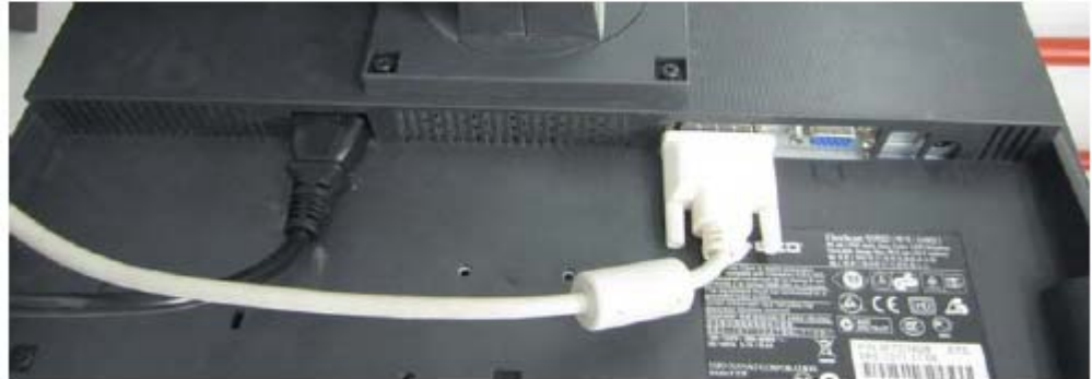
Figure 2-18 Video Cable and Power Cable for LCD Monitor
