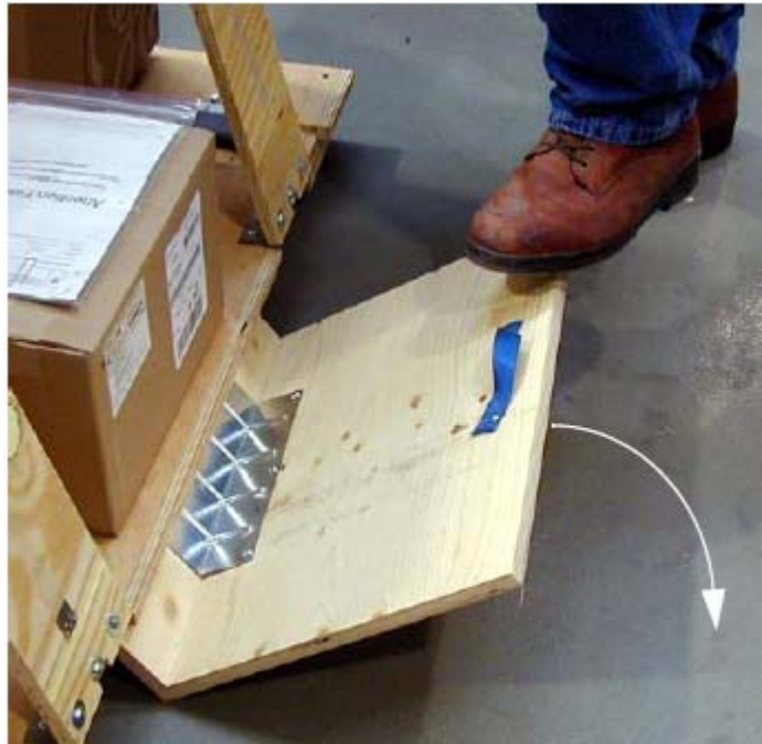
Figure 2-7 Step-Board Used to Raise Front Edge of Skid
