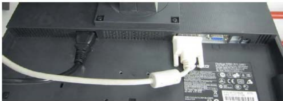
Figure 2-17 Video Cable and Power Cable for LCD Monitor
