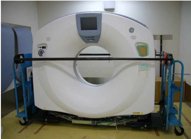
Figure 14-1 Gantry with Shipping Dollies and Side Rails
