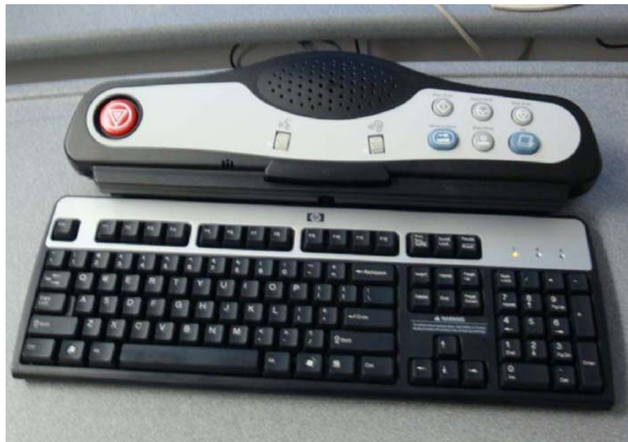
Figure 2-5 SCIM connected to the keyboard with the US English tilt overlay installed
