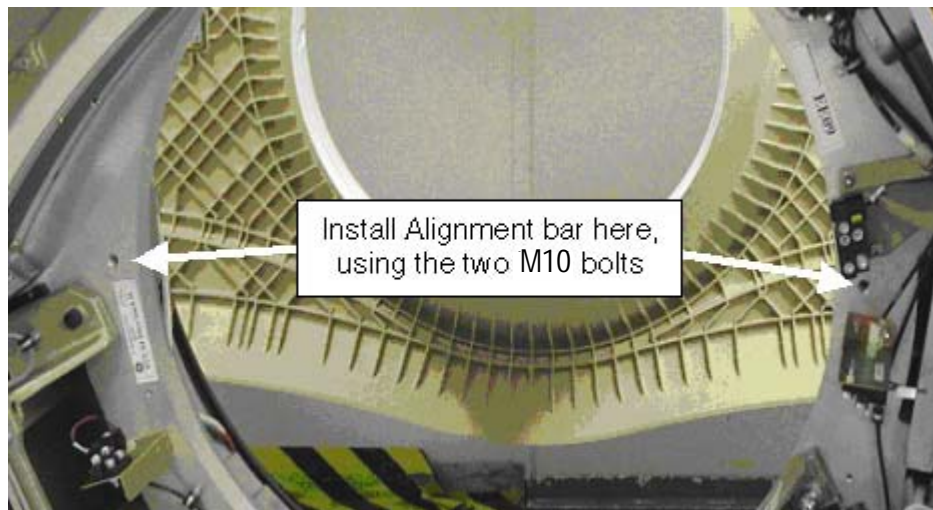
Figure 1-21 Alignment Bar Installation Location
