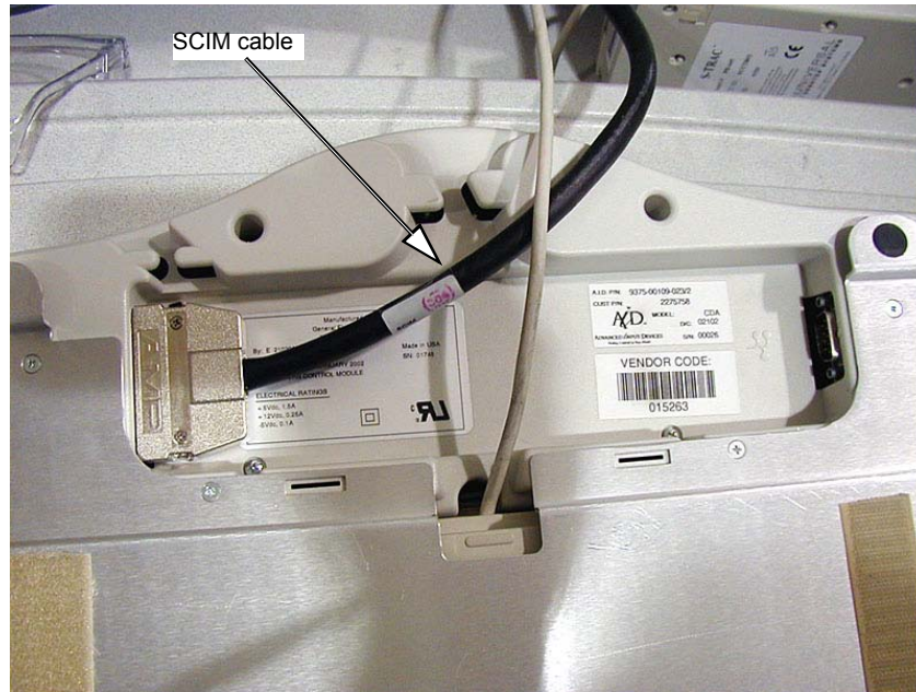
Figure 2-4 SCIM bottom, showing cables and keyboard mounting bracket
