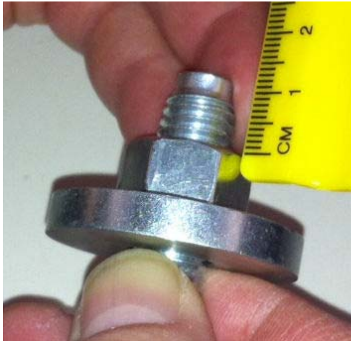
Figure 1-57 Anchor Preparation-set nut at 13.0 mm
