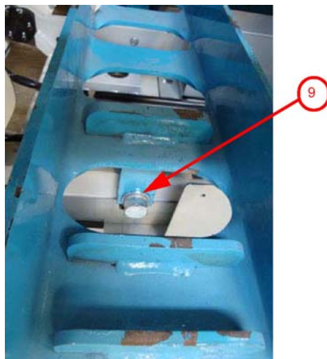
Figure 1-64 Close-up of table base connection
