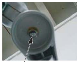
Junction Bolt (Notice the direction during reconfiguration)
