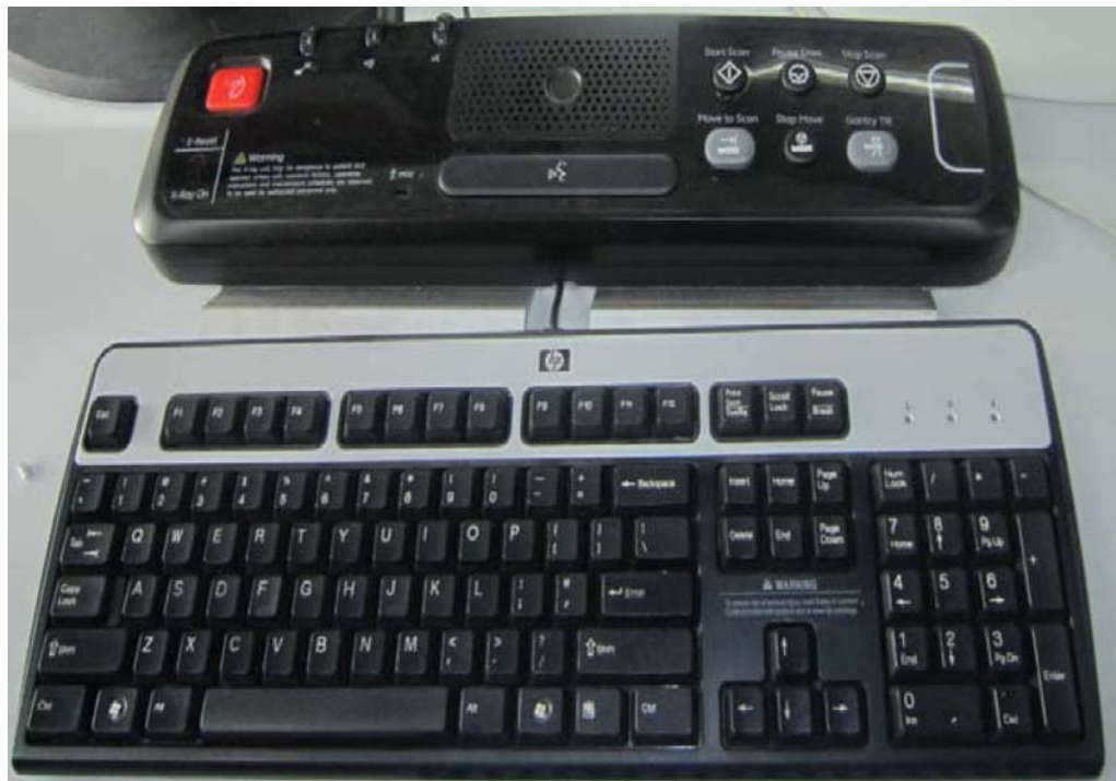
Figure 2-7 GSCB connected to the keyboard with the US English tilt overlay installed
