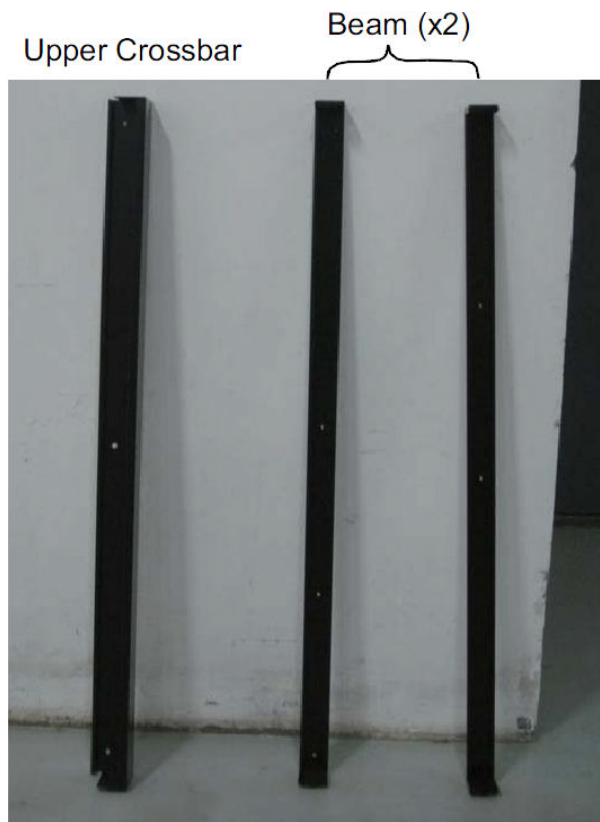
Figure D-2 Crossbar and Beams
