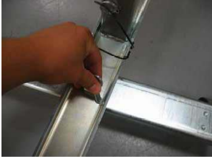
Figure A-10 Place Pin to Secure Feet
