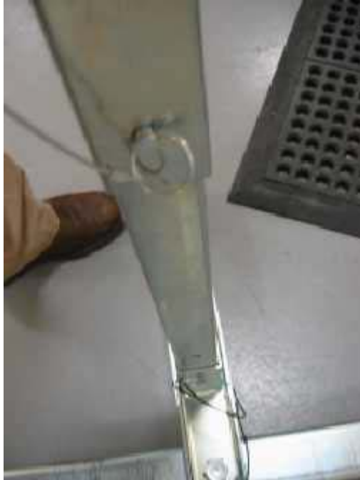
Figure A-12 Secure Bracket with Pin
