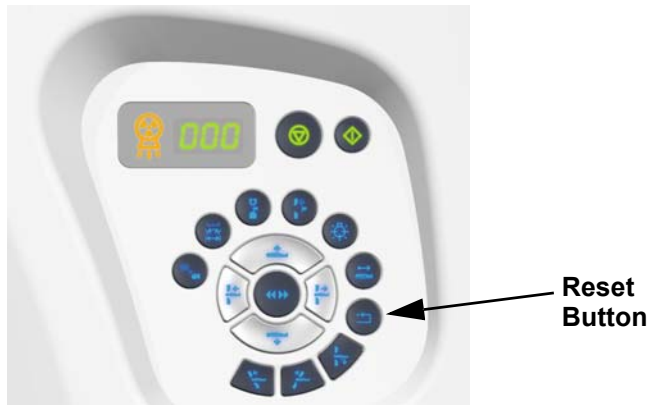
Figure 4-21 Reset buttons on Gantry Switch
