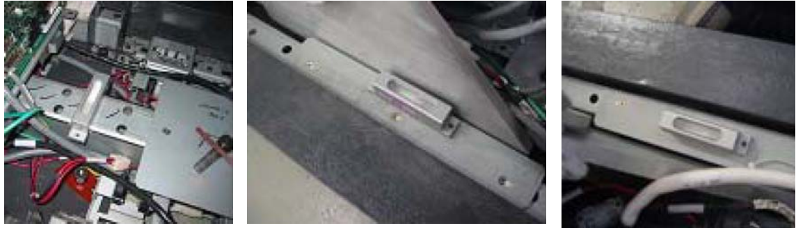
Figure 1-48 Place Bubble Level
