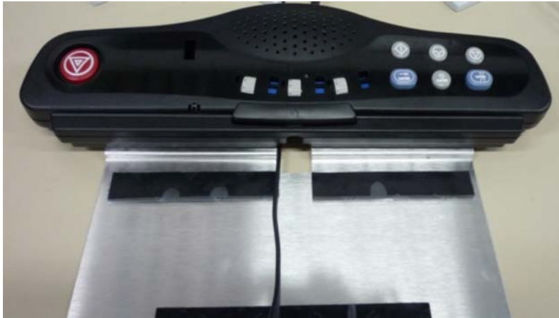
Figure 2-3 SCIM control with keyboard cable routed through SCIM (actual components may vary in style)
