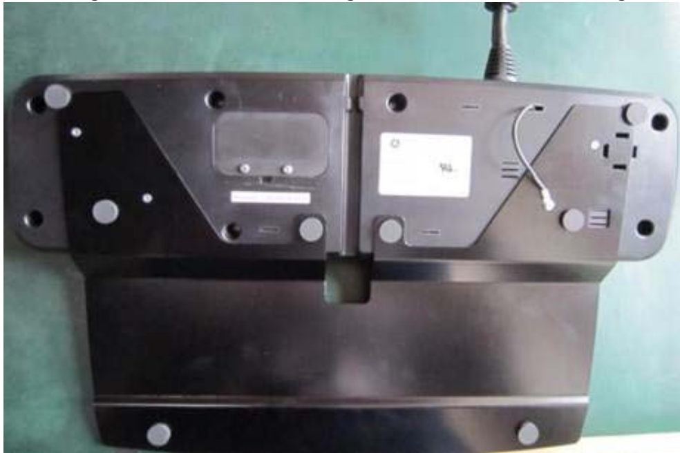
Figure 2-11 Metal Plate Installing and Ground Cable Connecting
