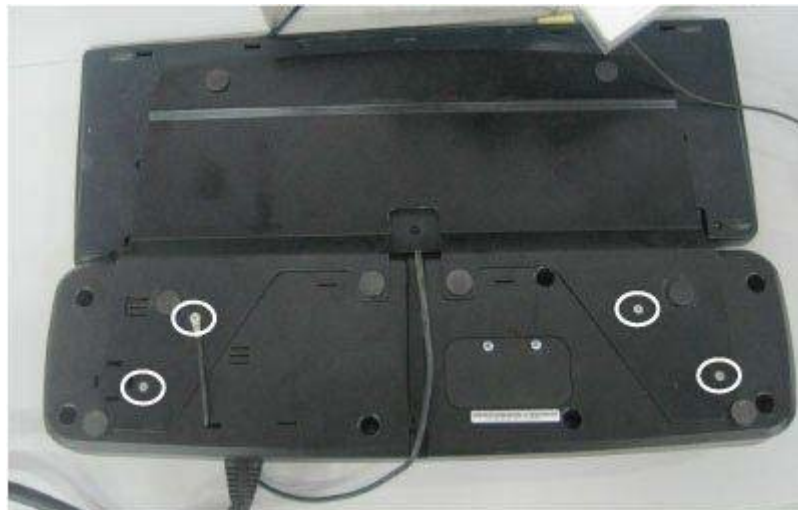
Figure 2-2 Metal Plate Removal
