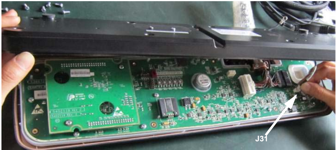
Figure 2-4 Disconnect E-Stop Cable Connector
