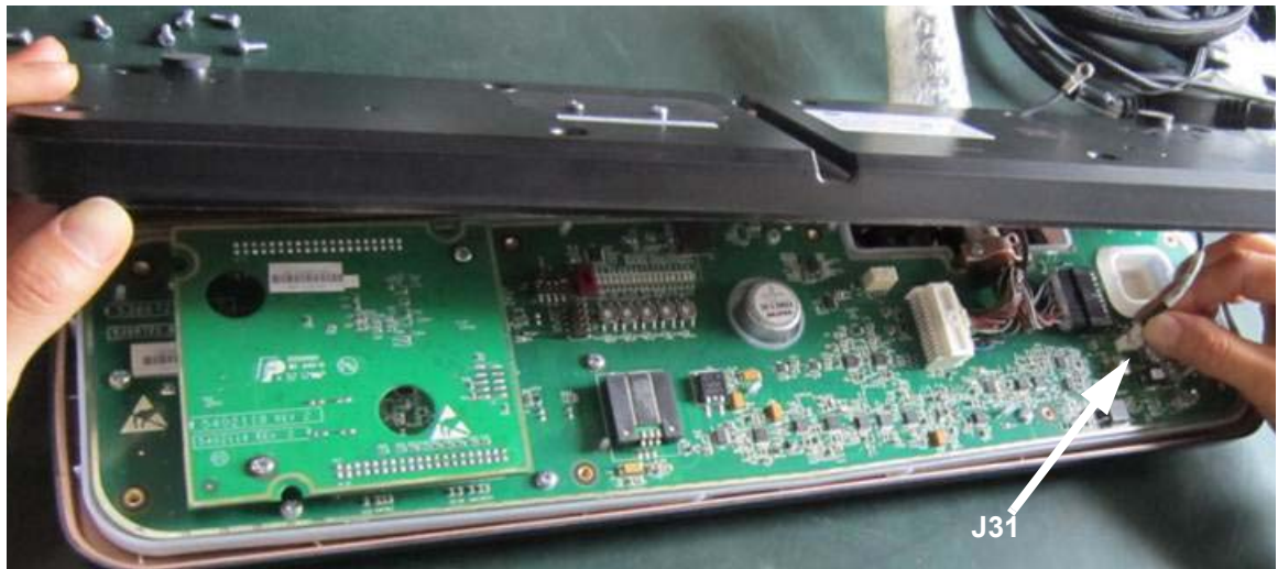
Figure 2-4 Disconnect E-Stop Cable Connector
