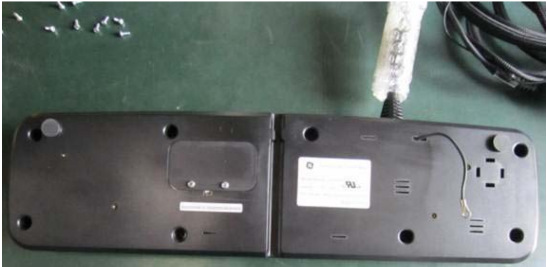
Figure 2-3 Remove Screws from GSCB Rear Cover
