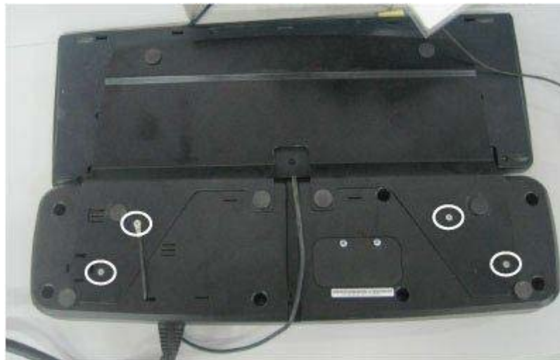
Figure 2-2 Metal Plate Removal
