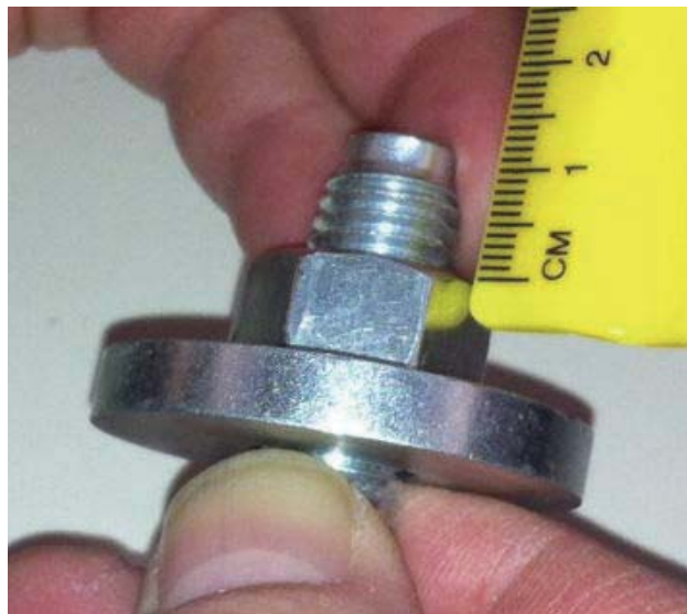
Figure 2-55 Anchor Preparation-set nut at 13.0 mm
