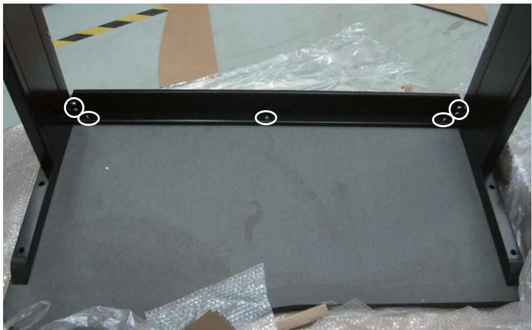
Figure B-26 Crossbar Installation
