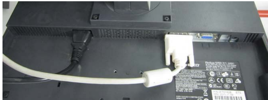
Figure 3-8 Video Cable and Power Cable
