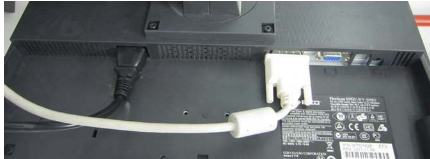
Figure 3-11 Video Cable and Power Cable
