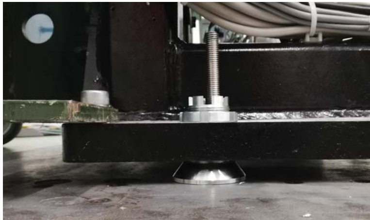
Figure 2-29 Lower the Gantry
