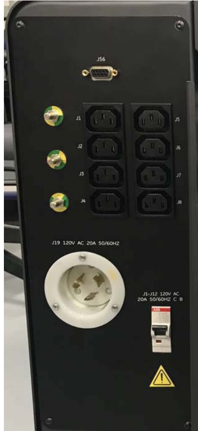
Figure 3-45 Open Console (Z8G4) AC Box Connections
