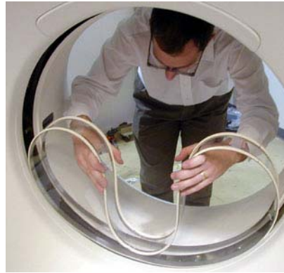
Figure A-2 Installing the mylar window
