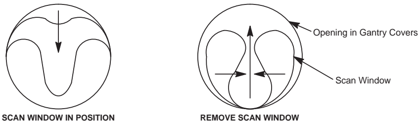
Figure A-1 Scan Window Removal
