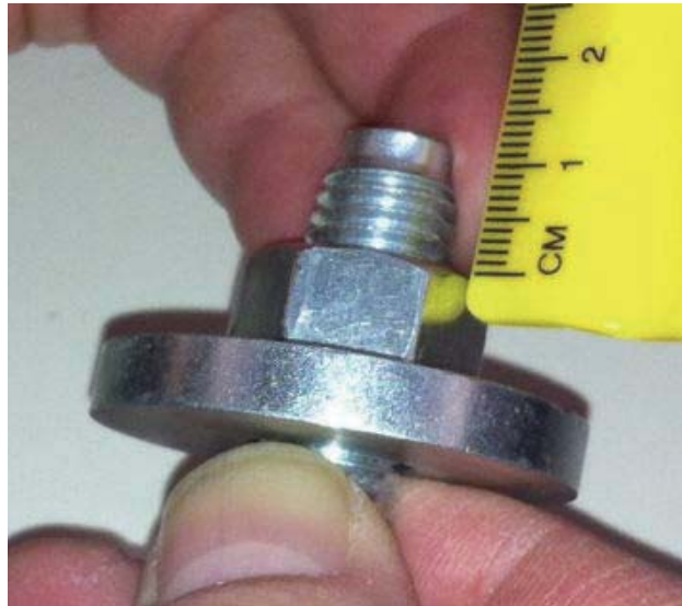
Figure 1-41 Anchor Preparation-set nut at 13.0 mm
