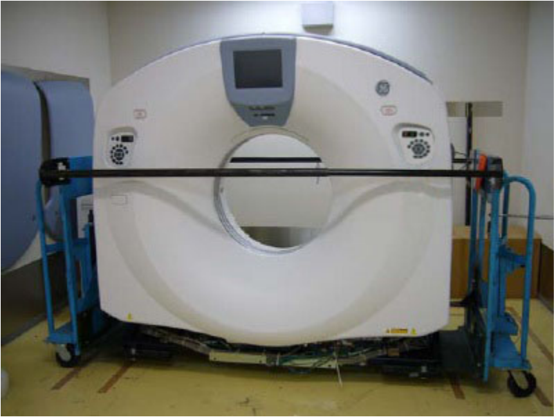
Figure 14-1 Gantry Shipping Dollies with Side Rails
