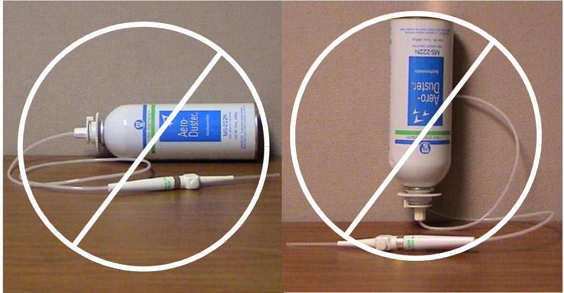
Figure 1-5 Wrong Angles will generate Liquid Spray
