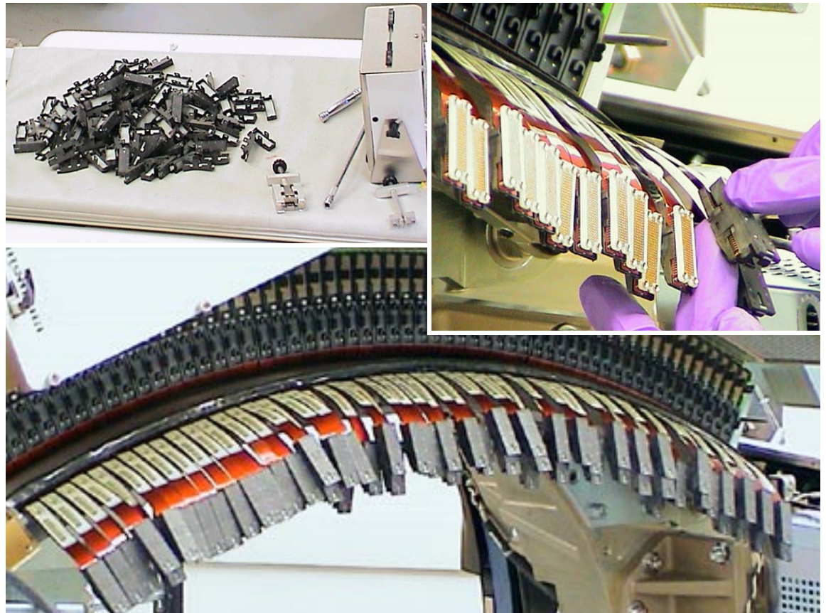
Figure 1-14 16 Slice Hardware, Flex Removal and ESD Boot Installation
