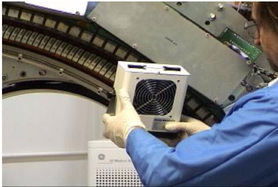
Figure 1-9 Using the Ionizing Fan to dissipate charge at the DDIF
