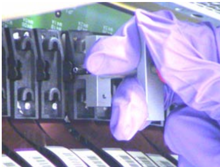
Figure 1-12 16 Slice Flex Removal Tool Usage
