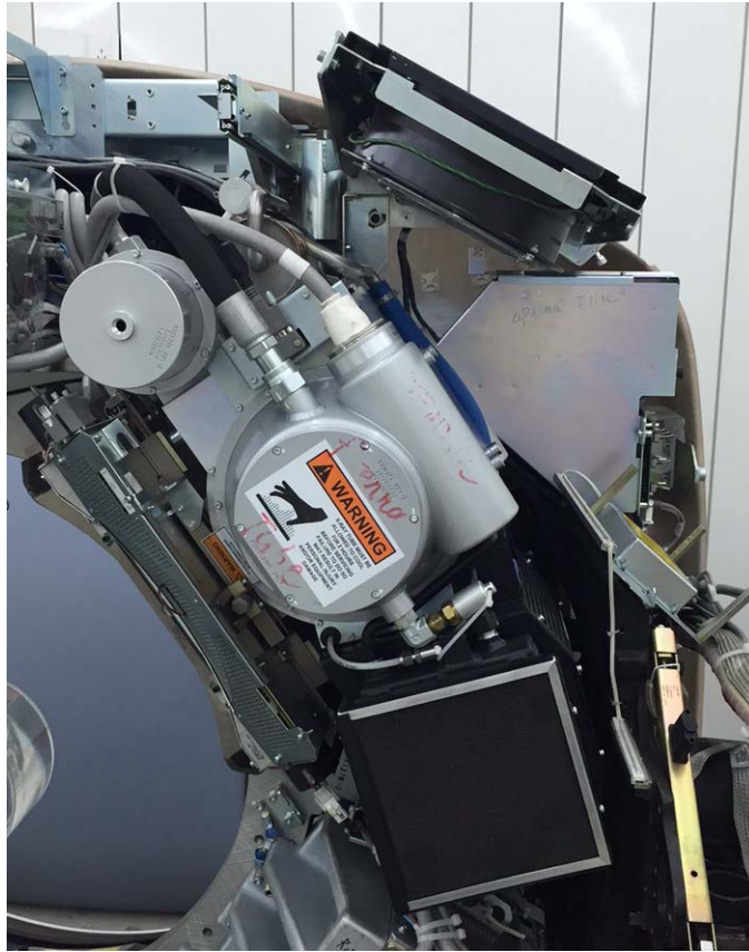
Figure 2-17 Tube Angle to Loosen and Torque M12 Screws
