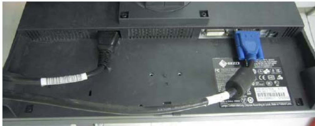
Figure 2-10 Video Cable and Power Cable for Image Monitor
