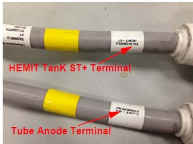
New Anode HV Cable Terminals
