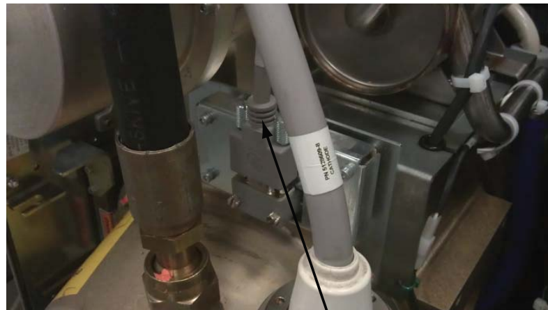
Figure 2-50 Smart ID Cable Connection
