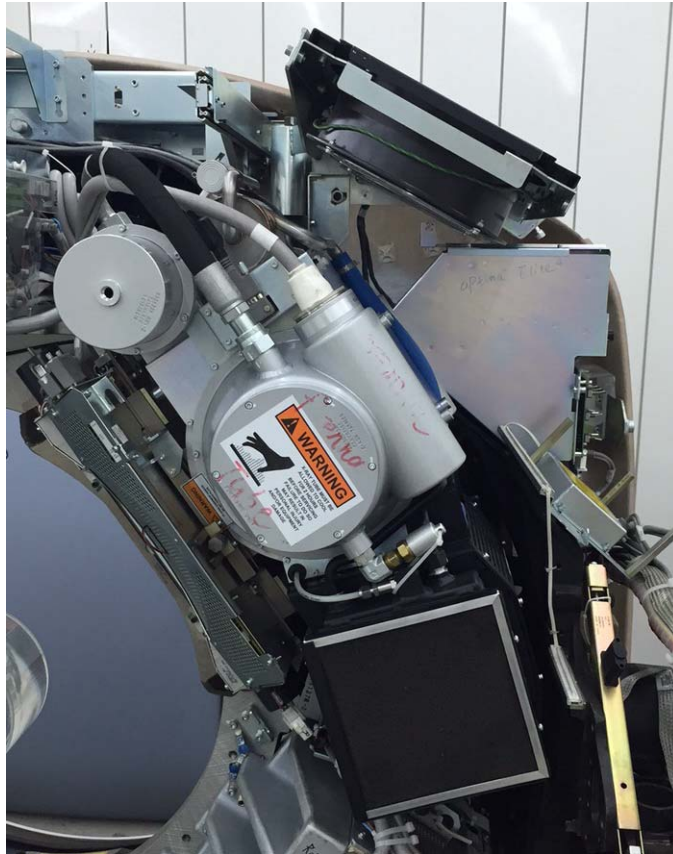
Figure 2-39 Tube Angle to Loosen and Torque M12 Screws
