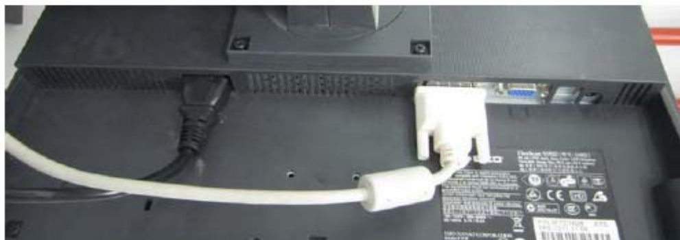
Figure 2-10 Video Cable and Power Cable for LCD Monitor
