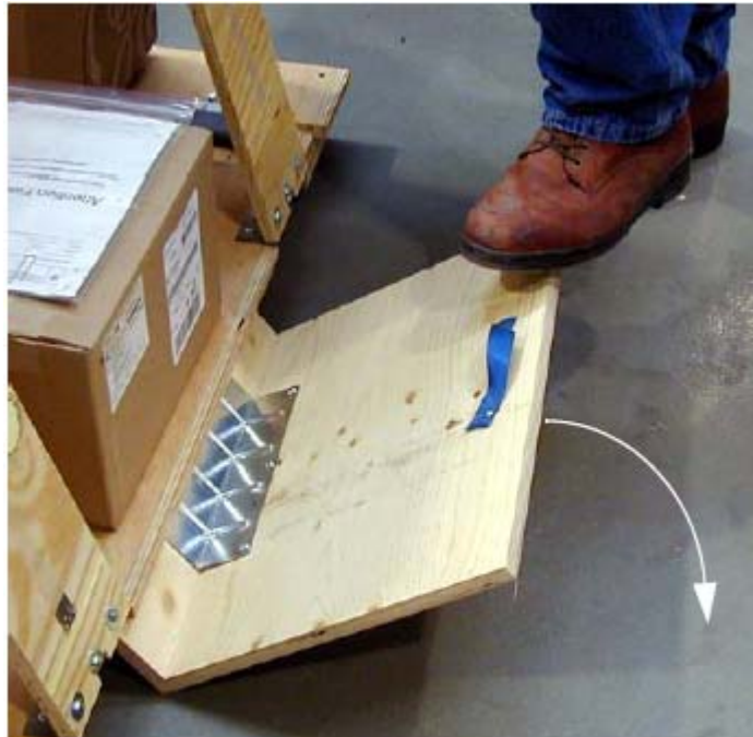
Figure 2-3 Step-Board Used to Raise Front Edge of Skid
