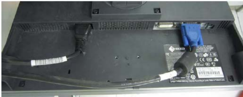
Figure 2-22 Video Cable and Power Cable for Display Monitor
