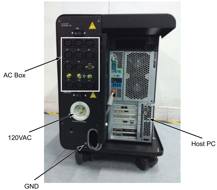
Figure 2-19 OpenOC16 Console Rear View
