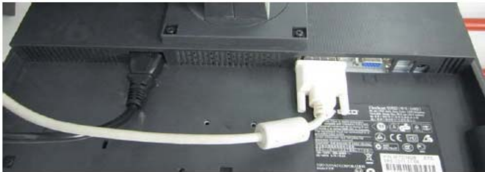
Figure 2-21 Video Cable and Power Cable for Scan Monitor
