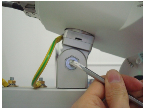
Figure 10: Fix the single camera position
