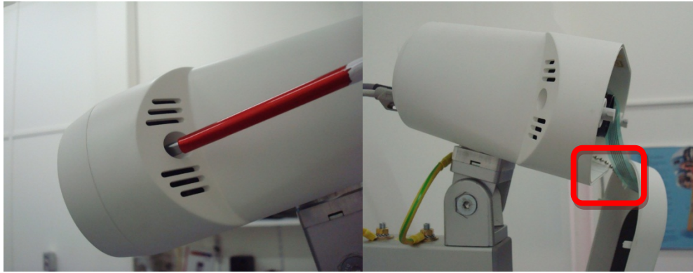
Figure 7: Remove Front Cover of the Single Camera
