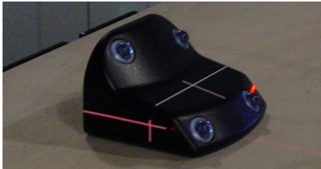
Figure 6: Align reflector block to the isocenter
