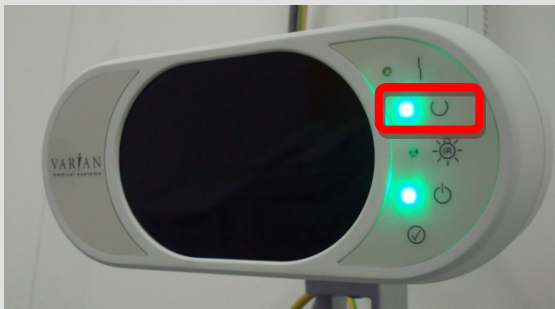
Figure 17: Tool Detected LED
