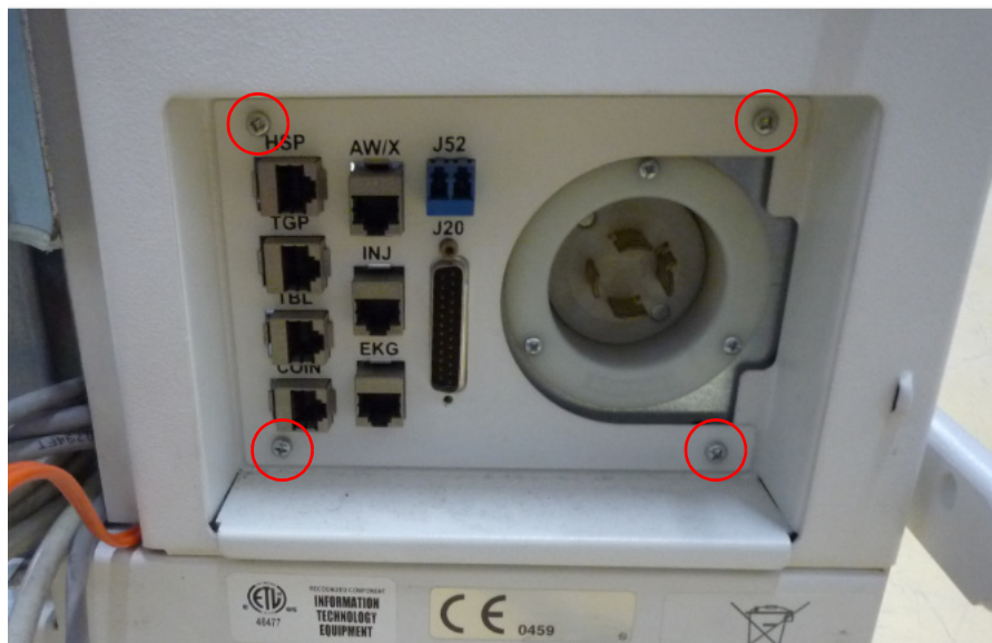
Figure 2-31 Rear Bulkhead Removal
