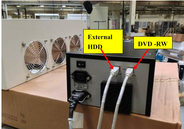
Figure 2-37 Peripheral Tower Connection
