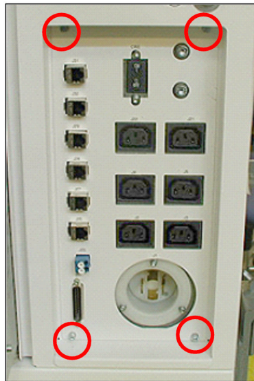
Figure 2-28 Rear Bulkhead Removal
