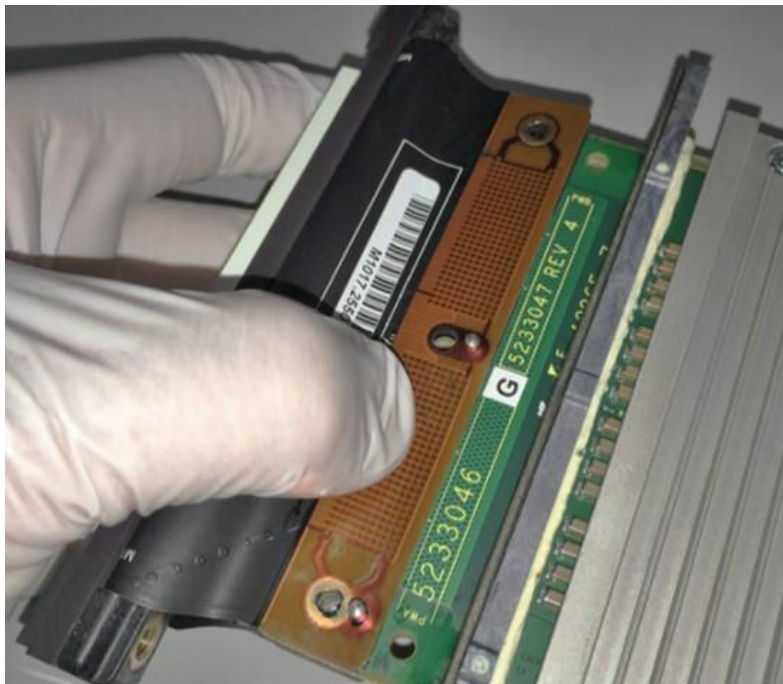
Figure 2-28 Top Clamp Reinstalled (Halo example)
