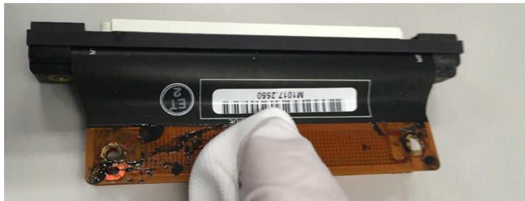
Figure 2-19 Cleaning of outer side of Flex (Halo example)
