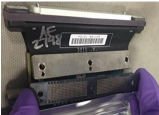
Figure 2-6 Top Interposer Removal (except for Saturn Outer module)
