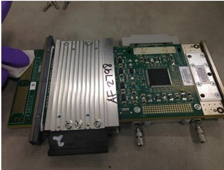
Figure 2-17 A/D Sandwich contact pads cleaning (Halo example)
