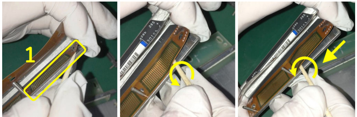
Figure 2-11 Flex separated from Bottom Clamp, area without alignment pin
