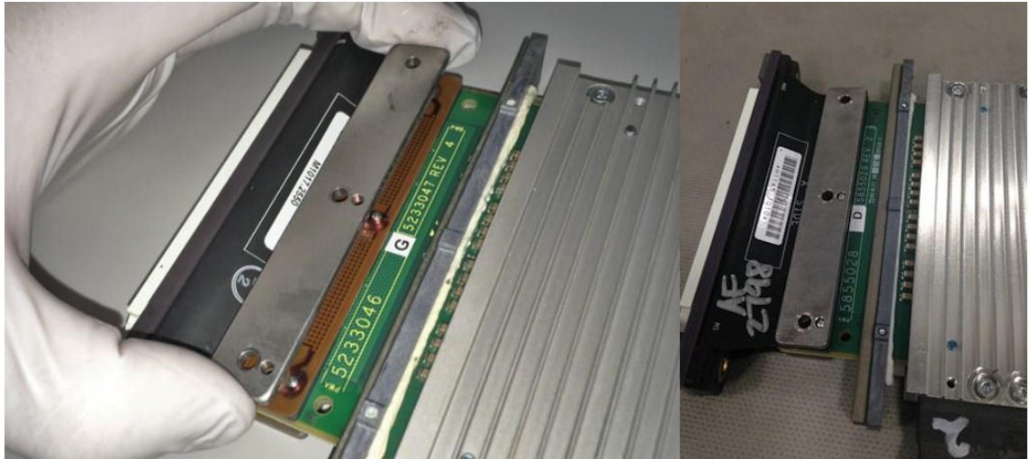
Figure 2-29 Top Clamp Reinstalled (Halo example)
