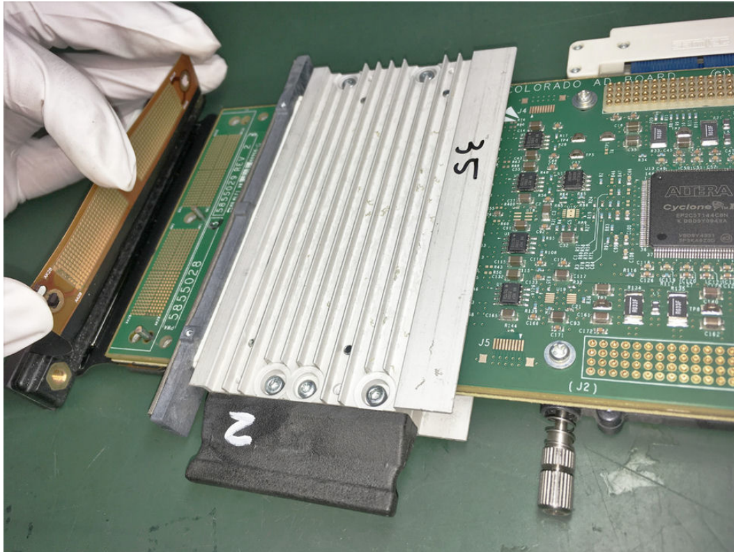
Figure 2-25 AD Sandwich Aligned to Bottom Clamp
