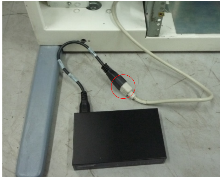
Figure 2-25 Connect Power Plugs
