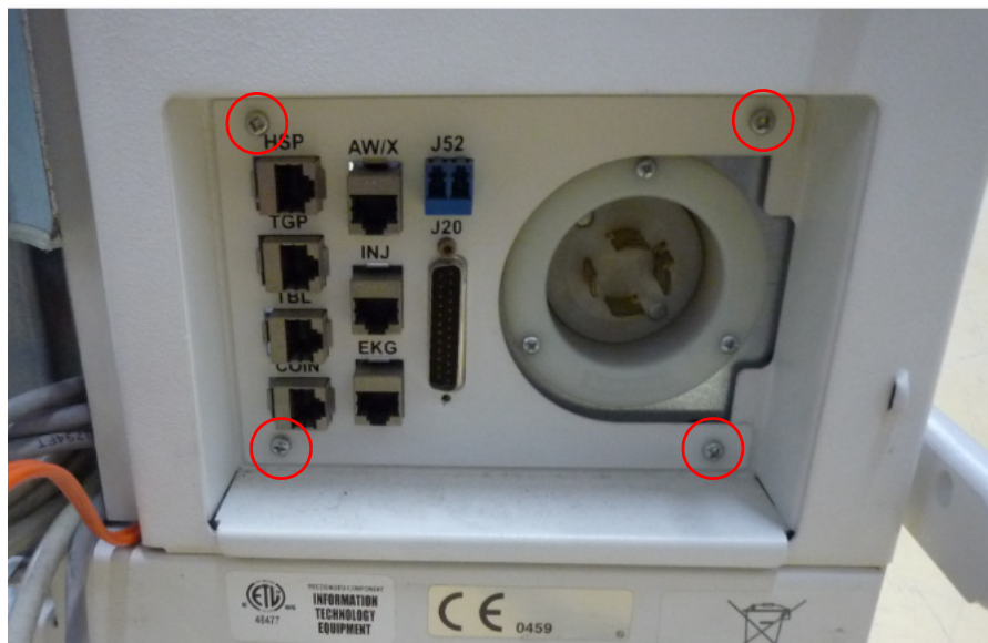
Figure 2-31 Rear Bulkhead Removal
