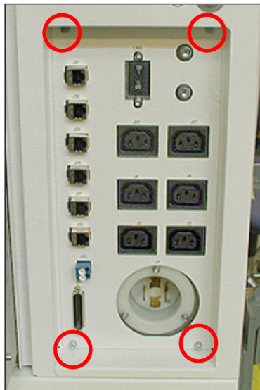
Figure 2-28 Rear Bulkhead Removal
