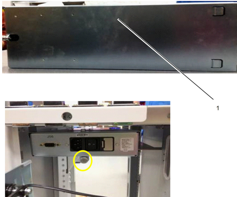
Figure 2-19 Install GSCB Console Power Box
