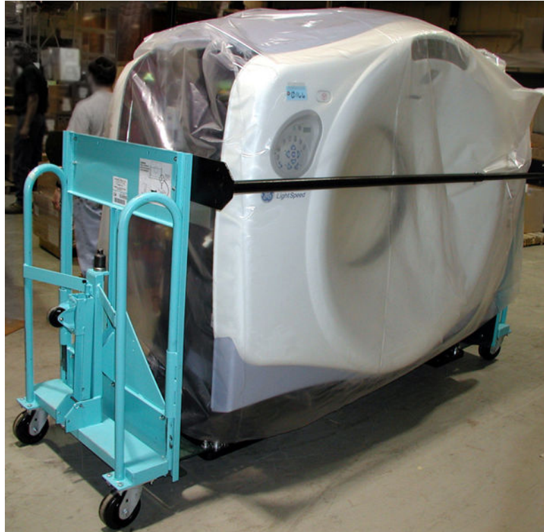
Illustration 14-1: Gantry with Shipping Dollies and Side Rails
