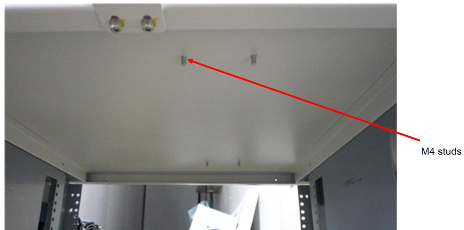
Figure 2-6 M4 Studs already built-in (example)
