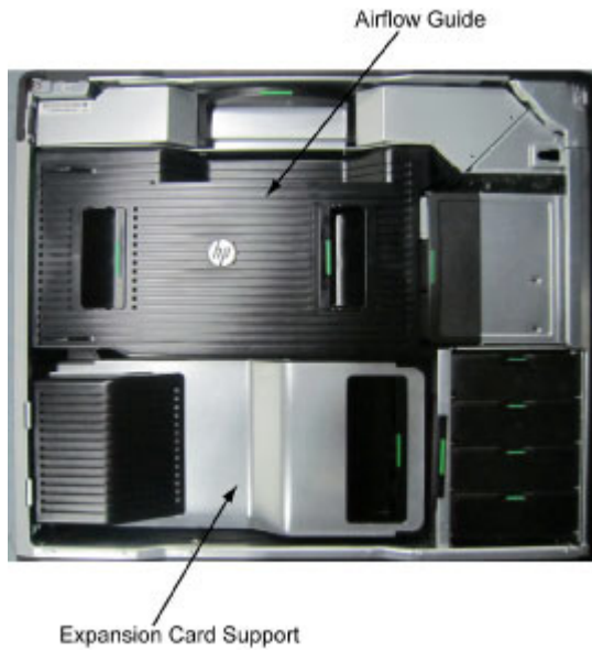
Figure 2-14 Z820 Airflow Guide and Expansion Card Support
