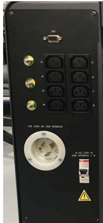
Figure 2-8 OpenOC with Z8G4 AC Box Assignments
