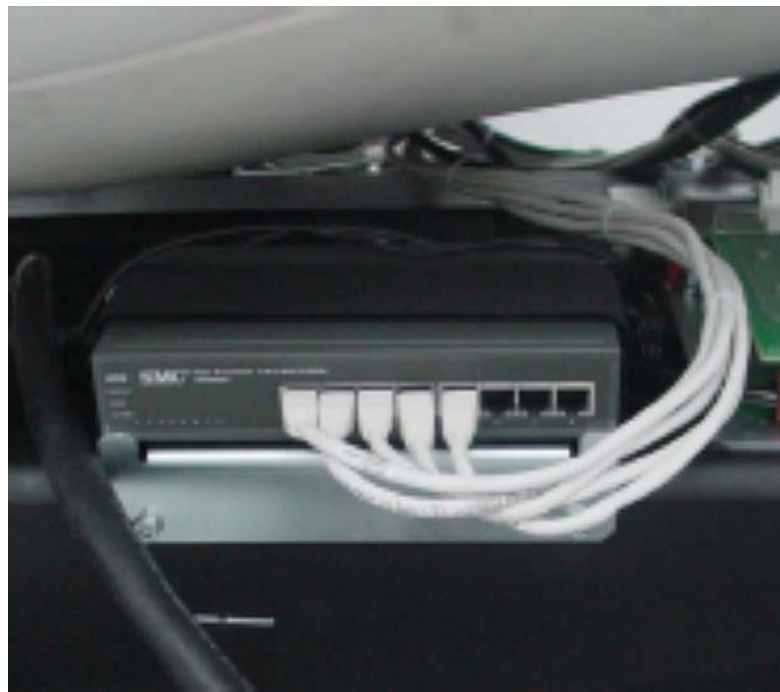
Figure 1-17 Cable Connection to LAN Switch
