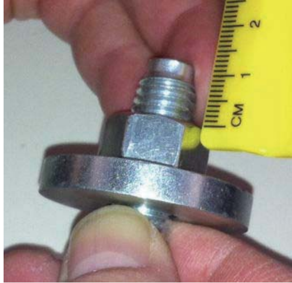
Figure 1-62 Anchor Preparation-set nut at 13.0 mm
