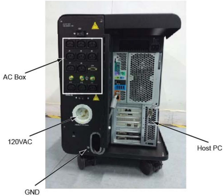
Figure 2-58 Open Console Rear View with AC BOX
