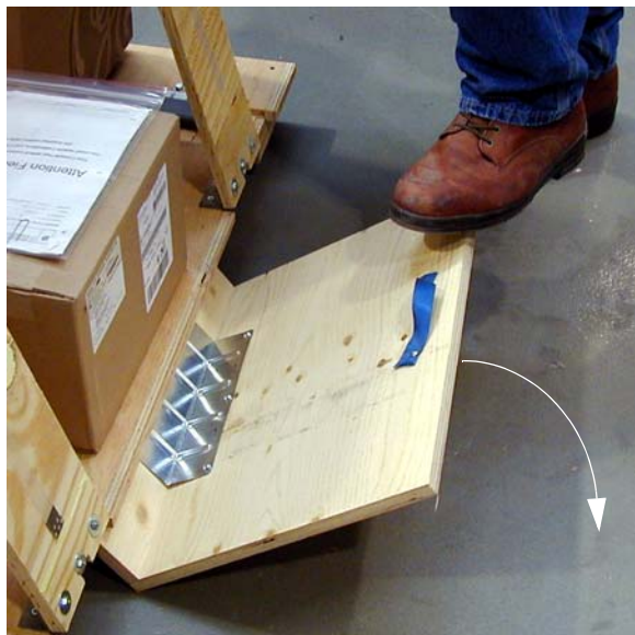
Figure 1-92 Step-board used to raise front edge of skid
