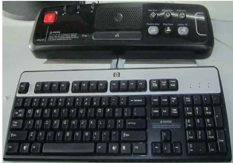
Figure 2-52 GSCB connected to the keyboard with the US English tilt overlay installed
