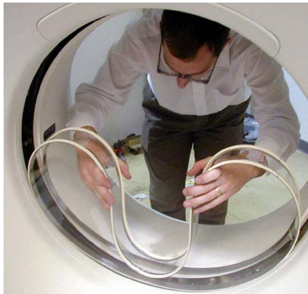
Figure A-23 Installing the mylar window
