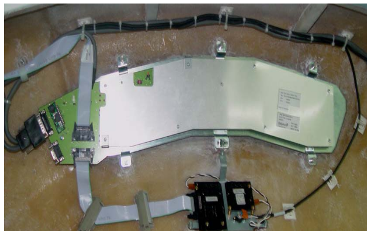
Figure A-13 Gantry Display Removal
