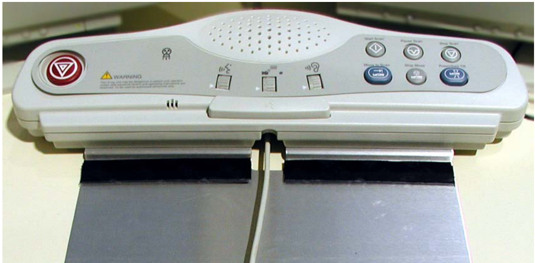
Figure 2-4 SCIM control with keyboard cable routed through SCIM
