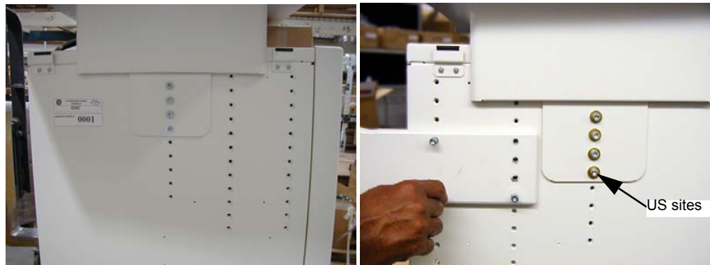
Figure 1-89 Global Console tabletop adjustments
