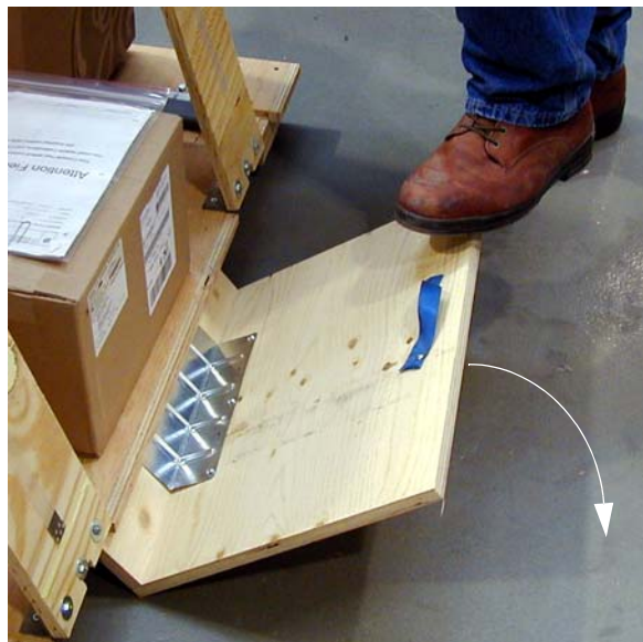
Figure 1-83 Step-board used to raise front edge of skid
