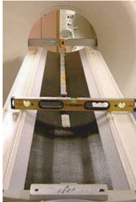
Figure 1-34 Table Level Alignment
