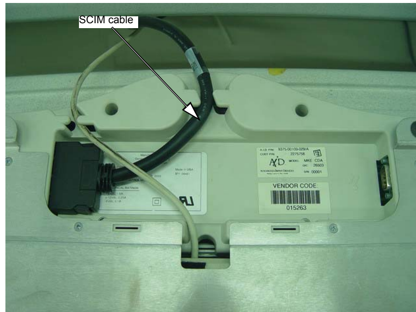
Figure 2-6 SCIM bottom, showing cables and keyboard mounting bracket
