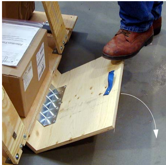
Figure 1-97 Step-board used to raise front edge of skid
