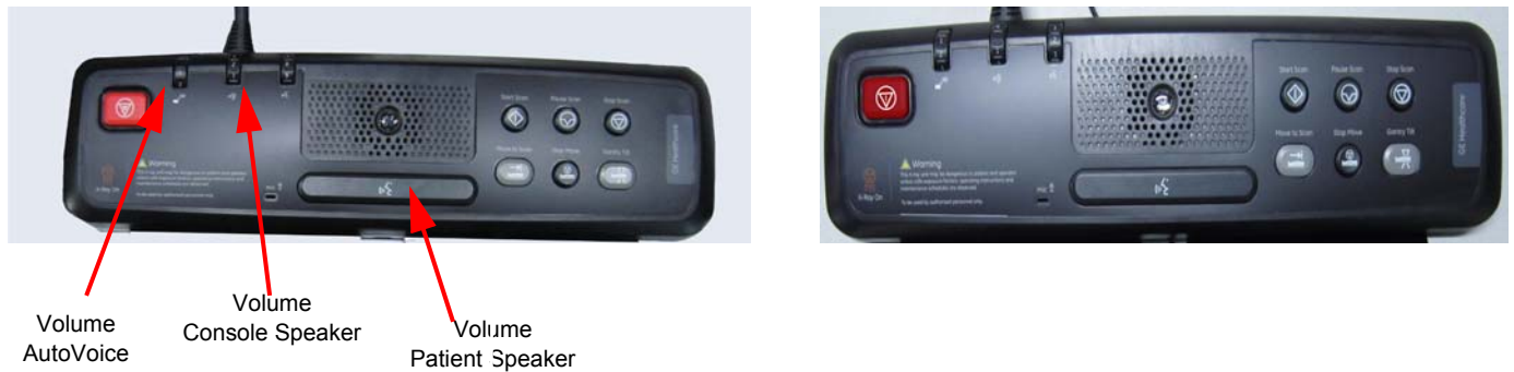
Figure 5-28GSCB Volume Controls on NIO16 Console
