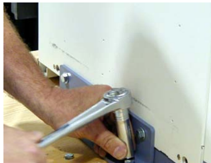
Figure 1-85 Removing the Seismic Brackets
