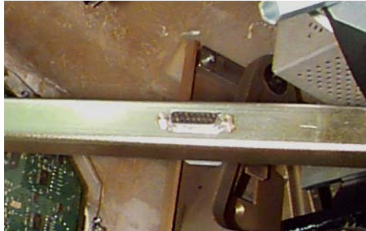
Figure A-17 Gantry Service Mode Cable Terminator
