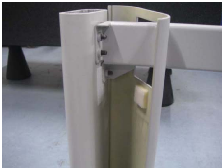
Figure B-17 Inner-Leg Cover and Adhesive Pad
