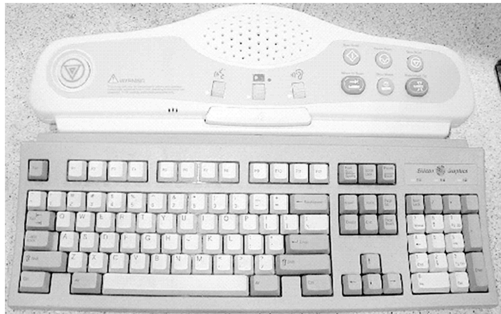
Figure 2-7 SCIM connected to the keyboard with the US English tilt overlay installed
