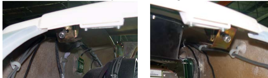
Figure A-4 Top Cover Mounting Screws
