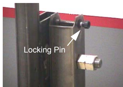
Figure A-11 releasing Front Cover Dolly Hinge
