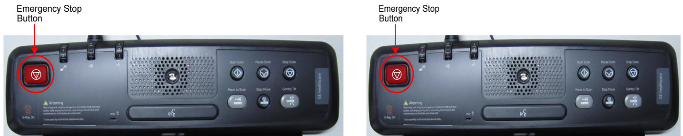
Figure 5-8 GSCB Emergency Stop Button on NIO16 Console
