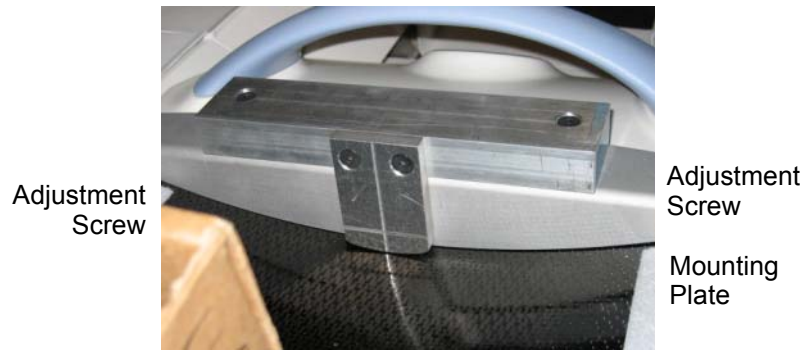
Figure 1-50 Cradle Rear Laser Alignment Tool
