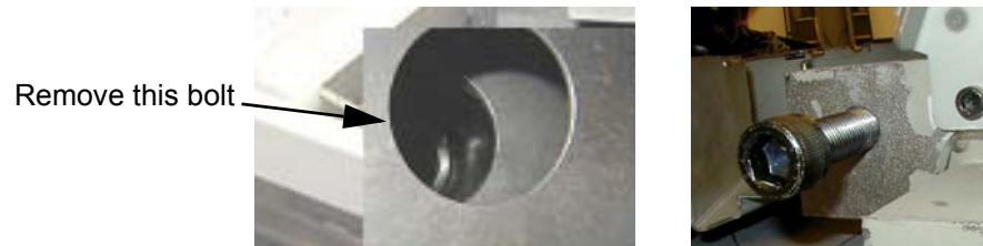
Figure 1-69 Dolly Side Panels - Front Bolt
