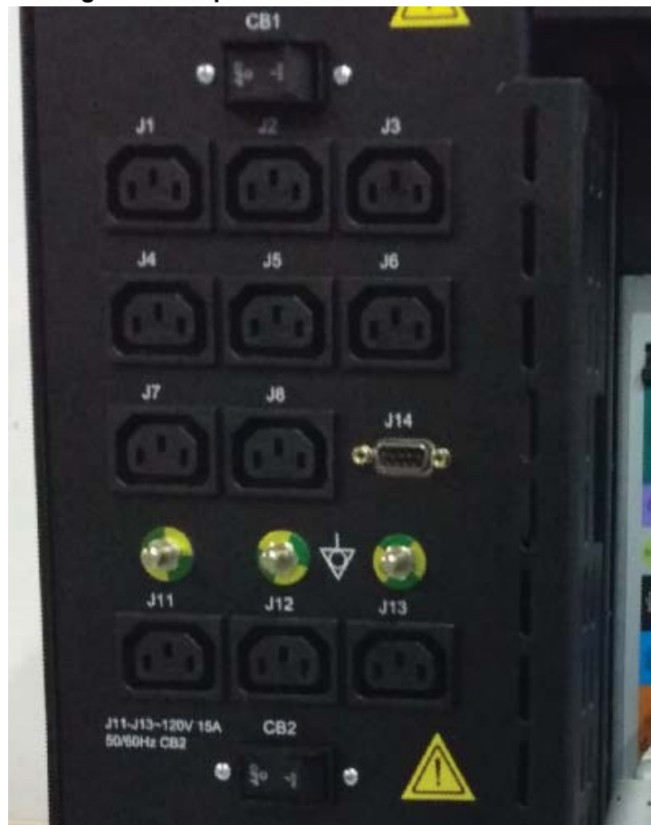
Figure 2-61 Open Console AC Box Connections
