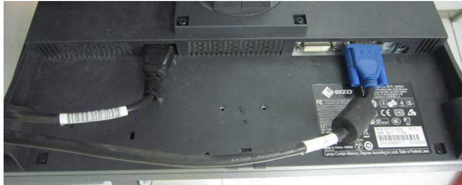
Figure 2-40 Video Cable and Power cable
