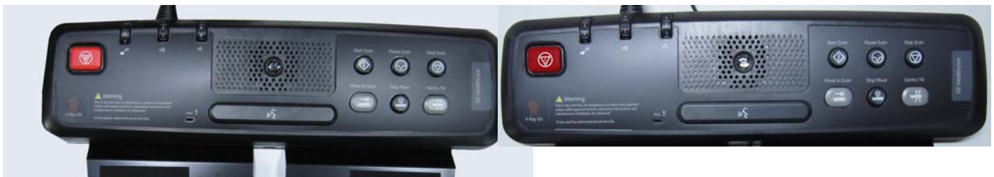
Figure 2-51 GSCB without E-Reset overlay
