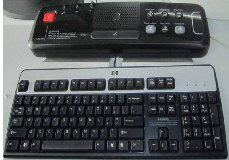
Figure 2-36 GSCB connected to the keyboard with the US English tilt overlay installed
