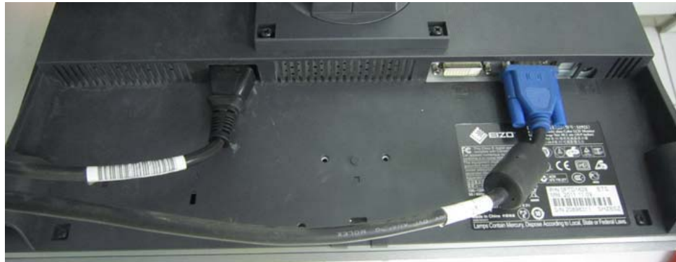
Figure 2-27 Video Cable and Power cable
