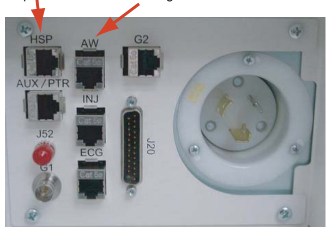
Figure 4-20 LCGOC/GOC4/AIO Console Rear Bulkhead
